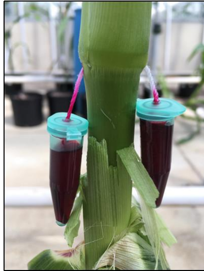
Figure 25. Experimental set-up for exogenous application experiments. A sewing needle was used to poke holes in the tops of two microcentrifuge tubes. The needle was poked through the maize stem at the specified location and the thread knotted inside both tubes. The tubes were filled with food dye and the hormone solution. Tubes were re-filled as needed for the duration of the experiment.
