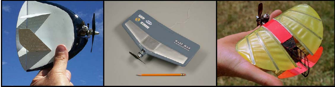
Figure 1.2: Fixed wing MAVs from left to right Trochoid developed by MLB, the Wasp developed at Aerovironment, and the flexible wing design developed at the University of Florida.
