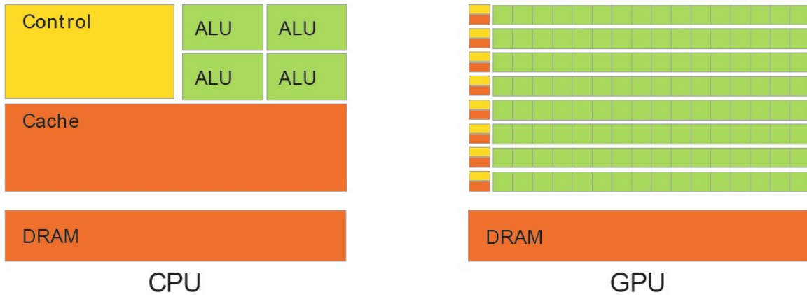
Figure 1.1: Comparison between General CPU and GPU (Image from Nvidia CUDA C programming guide [65]).
