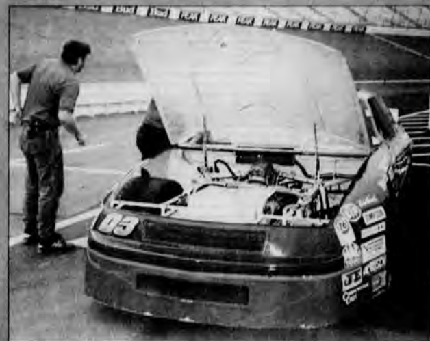
The 1994 Chevy Lumina's 274 cu. in. Buick V-6 delivers 490 horsepower and exceeds road speeds of 170 mph.
