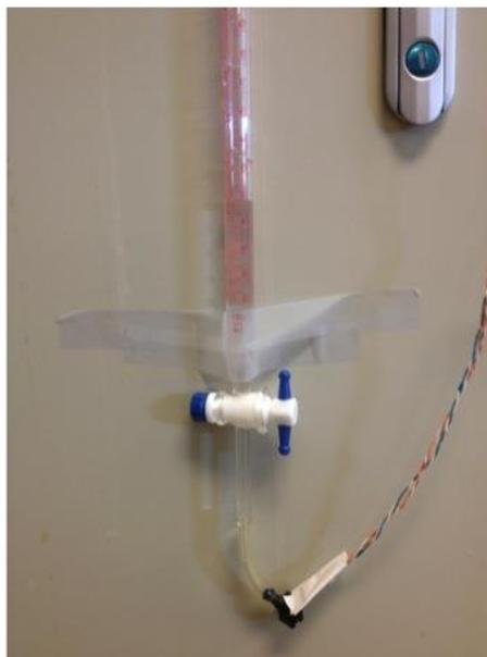
**Figure 2.4 Use of a water-filled burette to calibrate the pressure sensors using a Labview program**
