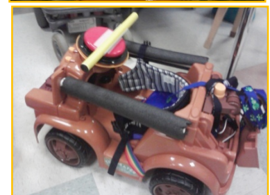
Figure 1 Ride on Toy Car. Bottom view shows the typical modifications of a PVC roll cage and large red switch with a yellow
