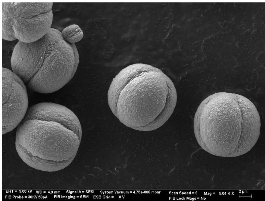
Figure B.7: SEM image of [B]ZSM-5 (F-1)
