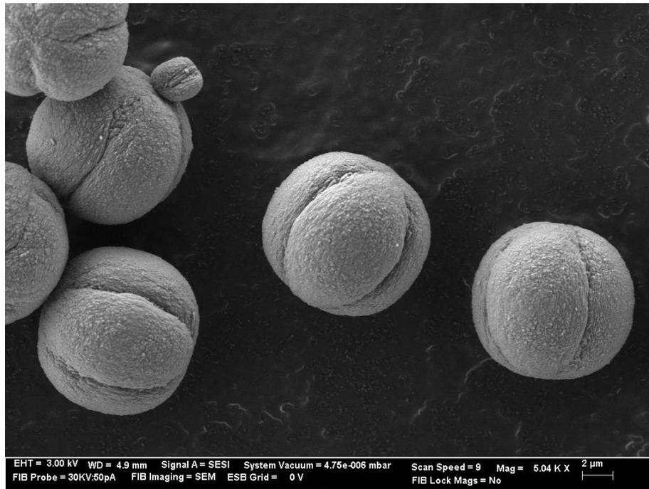
Figure 4.1: SEM image of [B]ZSM-5 (OH-1) (*top*) and [B]ZSM-5 (F-1) (*bottom*)
