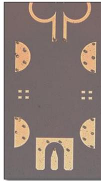
Figure 5.4: Post-disconnection photodiode bond pad with resultant indentations.
