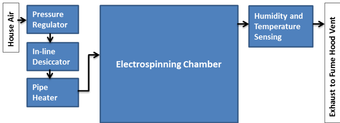
Figure 3.9 Schematic description of environmental process controls in Mark III system.
