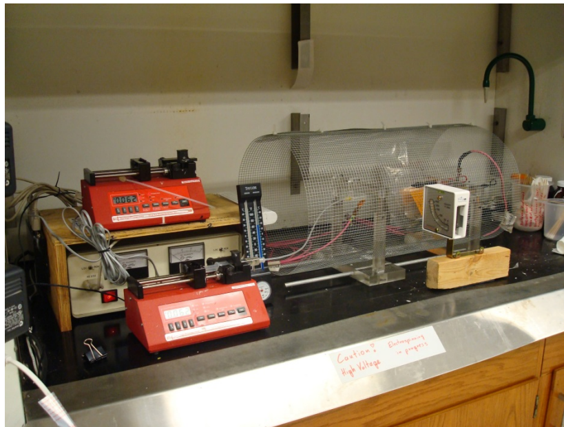
Figure A.3 Mark II electrospinning apparatus with Faraday cage
