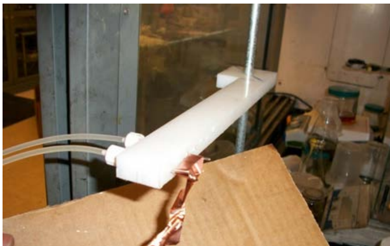
Figure A.1 Mark I, very rudimentary electrospinning apparatus
