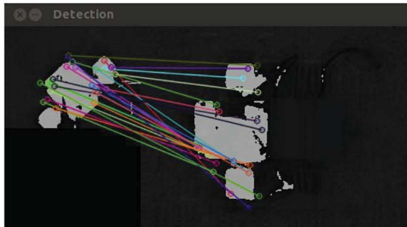
**Figure 7.7:** The hue part of the incoming frame (left) and the template image (right). The matched SURF features between two images are plotted as small dots linked by lines.
