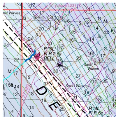
Figure 24 Location of chirp sub-bottom profile Ge01 indicated by thick dark blue trackline. Thick red lines indicate boundaries of DGS ID areas. DGS ID area Ge is the largest area shown in this image.
