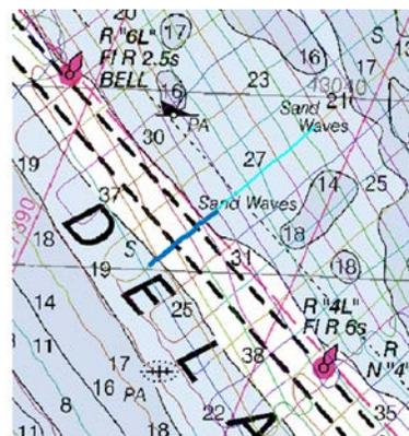
Figure 56 Location of chirp sub-bottom profile Ge06 indicated by thick dark blue trackline. DGS ID area Ge is the largest area shown in this image.
