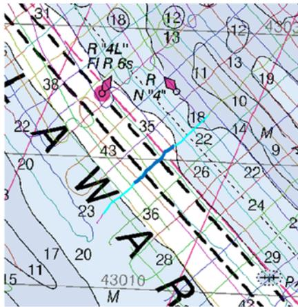
Figure 13 Location of chirp sub-bottom profile Ge15 indicated by thick dark blue trackline. DGS ID area Ge is the largest area shown in this image.
