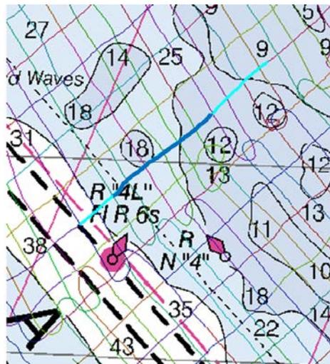
Figure 42 Location of chirp sub-bottom profile Ge27 indicated by thick dark blue trackline. DGS ID area Ge is the largest area shown in this image.
