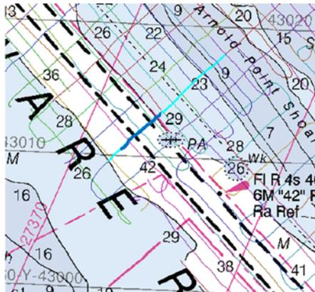
Figure 84 Location of chirp sub-bottom profile Ge20 indicated by thick dark blue trackline. DGS ID area Ge is the largest area shown in this image.
