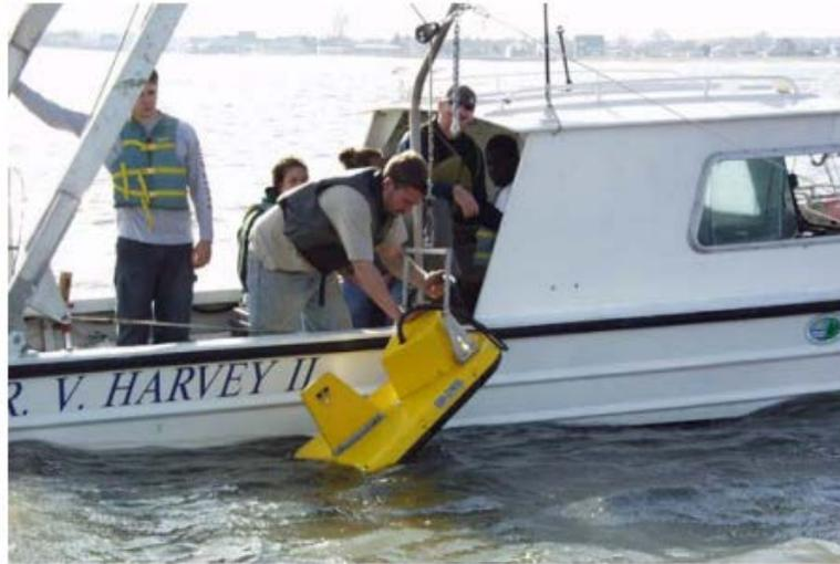
Figure 6 Deployment of the chirp towfish into the Delaware Estuary.
