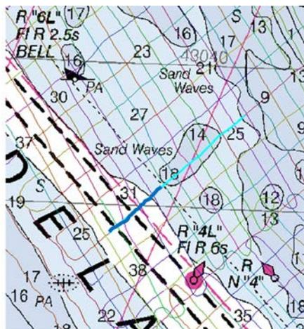
Figure 60 Location of chirp sub-bottom profile Ge08 indicated by thick dark blue trackline. DGS ID area Ge is the largest area shown in this image.
