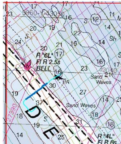
Figure 28 Location of chirp sub-bottom profile Ge03 indicated by thick dark blue trackline. Thick red lines indicate boundaries of DGS ID areas. DGS ID area Ge is the largest area shown in this image.
