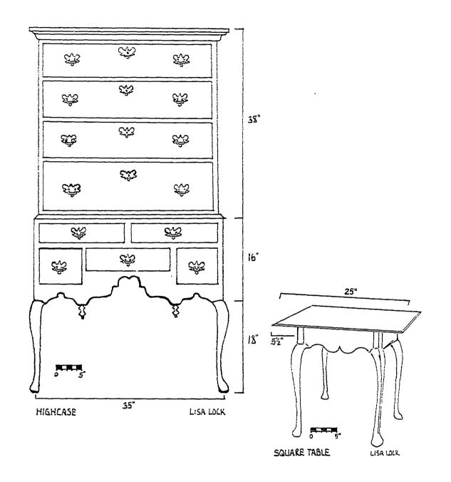
Figure 4.7. Interpretive drawings based on Doggett's furniture measurements. (Drawings by Lisa Lock.)
