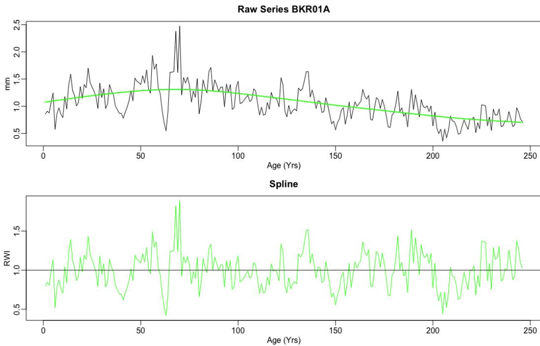
Figure 4: Example of a detrended ring-width series using the dplR package in R. The top plot represents raw ring-width measurements (mm) of a single core, shown by the black line, and is fitted with a cubic smoothing spline (green curve). The bottom plot shows the standardized ring-width indices (RWI) created by detrending using the cubic smoothing spline.
