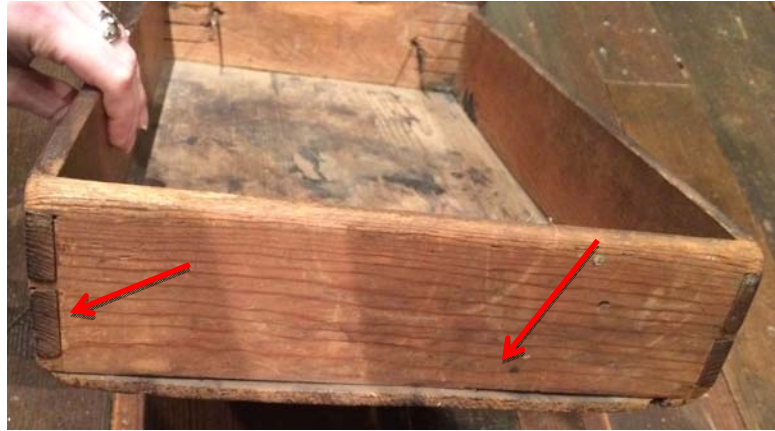
Figure 4.11 Detail, Figure 4.2. Central drawer, view from rear. Dressing table attributed to workshop of John Head. The red arrows indicate the extended bottom board and extended dovetails. Philadelphia, Pennsylvania, 1719–37. Courtesy Winterthur Museum, 1956.0038.143. Photo by author.
