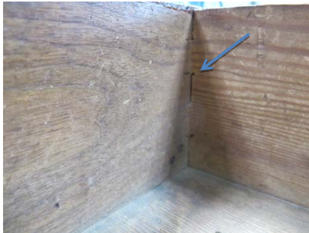
Figure 4.35 Detail, Figure 4.24. Chest of drawers made by William Beakes III. View of saw kerfs, front of smaller drawer seen from interior. Courtesy The Dietrich American Foundation. Photo by author.
