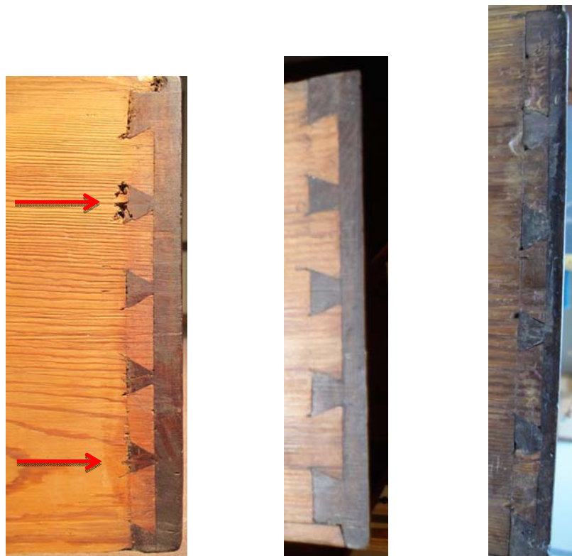
Figure 4.30 (left), Detail Figure 4.20; Figure 4.31, (center) Detail, Figure 4.22; Figure 4.32 (right), Detail, Figure 4.24. Chest of drawers made by William Beakes III., view of half-blind dovetail joint, front of drawer, with wedges in pins where indicated with red arrows (from left to right): Rocky Hill Collection; Private Collection; The Dietrich American Foundation. Drawers illustrated in Figures 4.30-4.32 do not all exhibit wedges in these photos, although wedges are found in other drawers of these chests. Photos by author.
