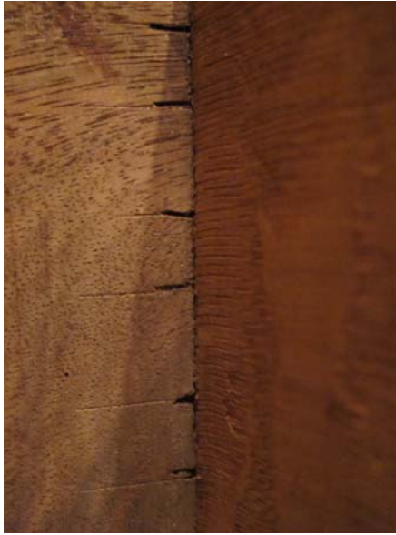
Figure 4.48 Detail, Figure 1.4. View of drawer interior with scribed lines and saw kerfs from cutting pins of dovetail joint. Chest on chest, dated 1738. Courtesy Winterthur Museum, 2009.0024, photo by author.
