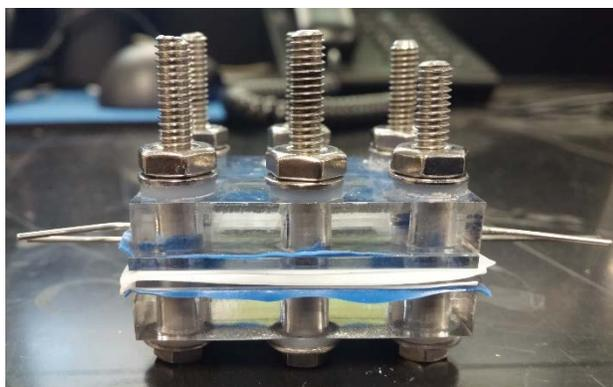
**Figure 5.1:** Constructed flow cell
