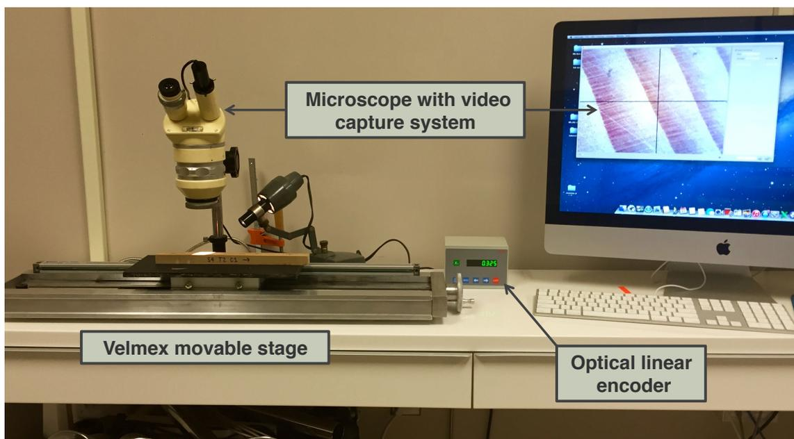
Figure 2: Ring-width measuring system
