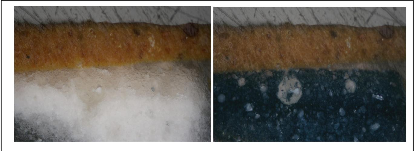
Figure 6.6 (left) and 6.7 (right): Paint cross-section (viewed at 50x magnification) of yellow ochre mixed with egg tempera atop a glue-gypsum ground before (left) and after (right) staining with Amido Black II. Note that only the glue-ground tested positive for the presence of protein.
