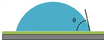
Figure 2-2. Schematic of a static sessile contact angle. The contact angle is determined by the balance of the interfacial tensions between the solid, liquid, and vapor phases.
