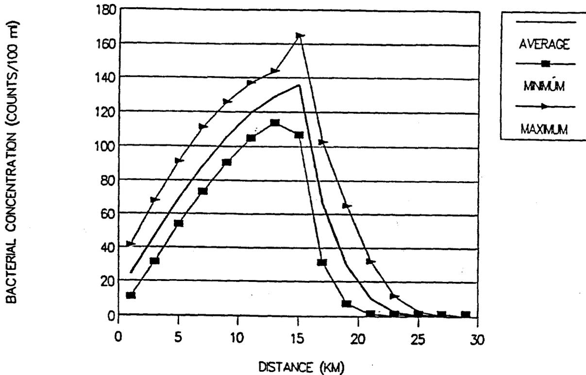
Figure 6-16. Predicted average, minimum and maximum bacterial concentrations for March versus distance from the mouth of the Trinity Estuary assuming no die-off.
