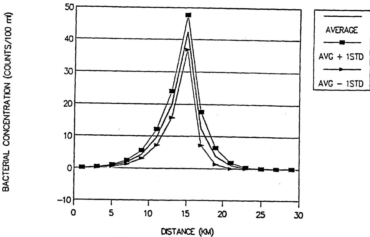
Figure 6-19. Predicted average bacterial concentrations, with their standard deviations, for March versus distance from the mouth of the Trinity Estuary, assuming a bacterial die-off rate of  $1.0 \text{ day}^{-1}$ .
