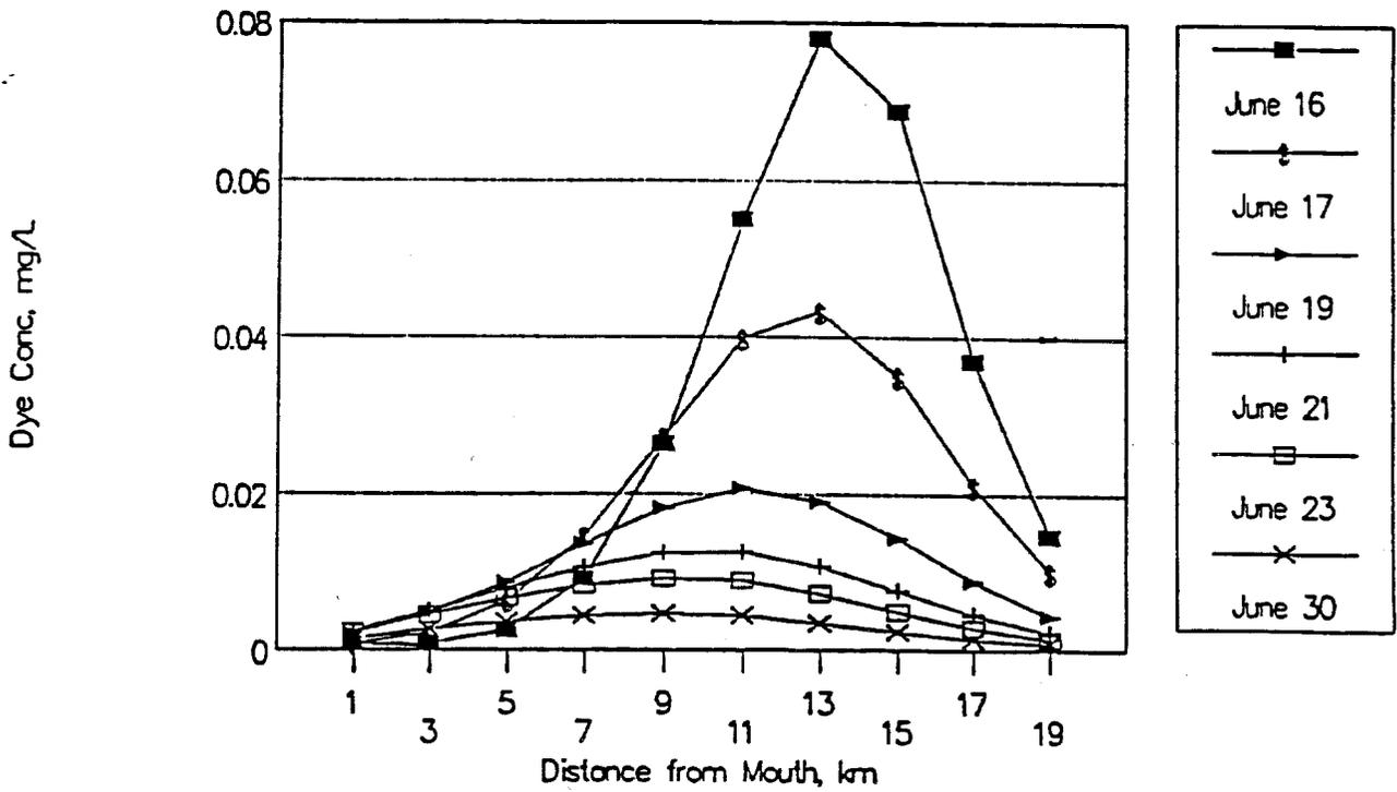
Figure 6-44. Deep Bay dye study center channel, surface.
