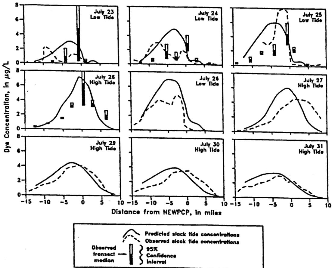
Figure 5-10. Observed and predicted dye concentrations [Ambrose (1987)].
