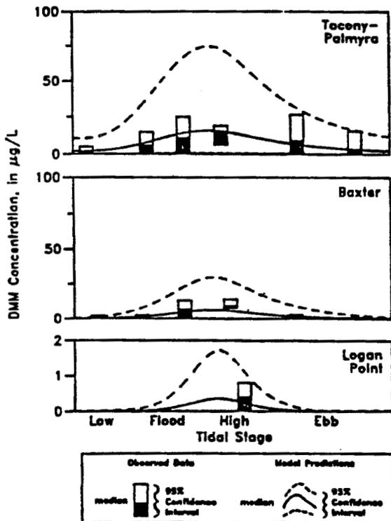
Figure 5-13. Observed and predicted DMM concentrations [Ambrose (1987)].
