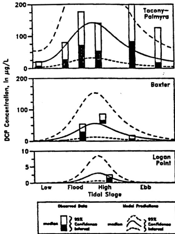
Figure 5-12. Observed and predicted DCP concentrations [Ambrose (1987)].
