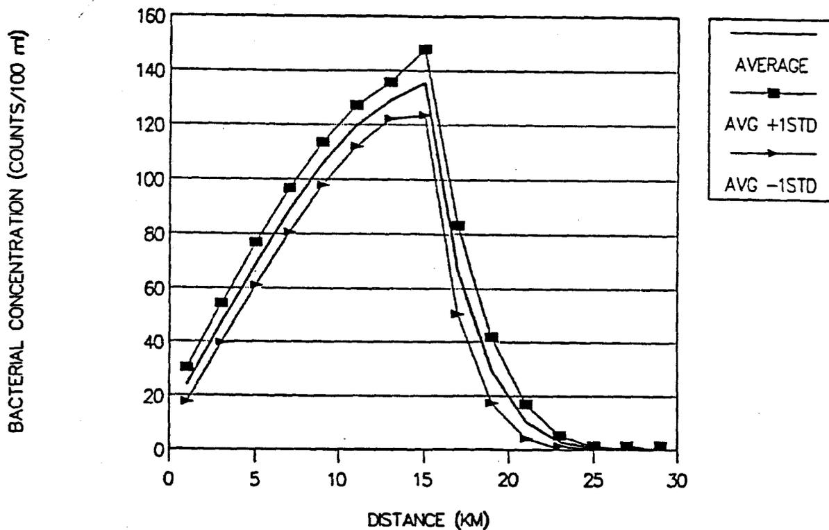
Figure 6-17. Predicted average bacterial concentrations during March, with standard deviations, versus distance from the mouth of the Trinity Estuary assuming no die-off.
