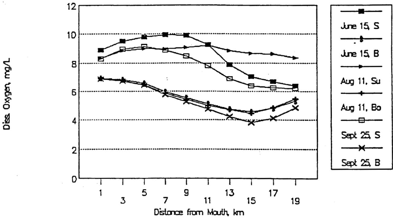
Figure 6-46. Deep Bay dissolved oxygen - June-Sept, surface and bottom.
