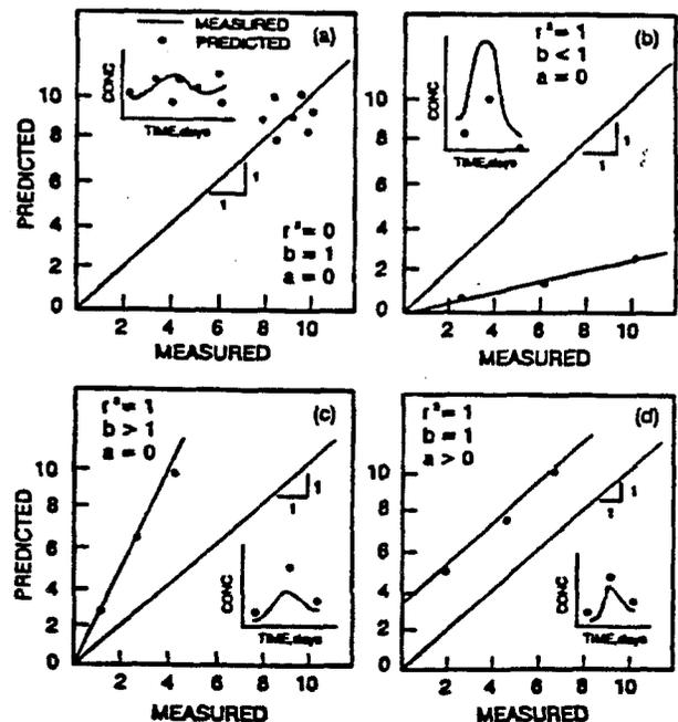
Figure 5-7. Types of bias and systematic error determined by regression analysis [(O'Connor (1979), Thomann (1982), and NCASI (1982)].
