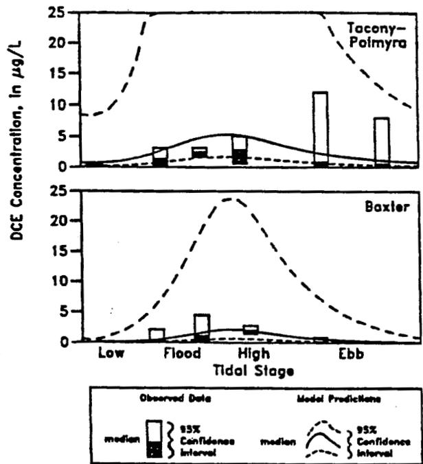
Figure 5-14. Observed and predicted DCE concentrations [Ambrose (1987)].
