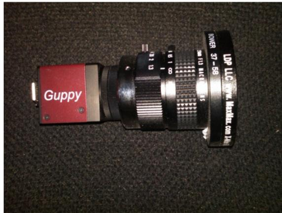
**Figure 2.6: Allied Vision Technologies: Guppy F-038C (NIR) with filter attached**
