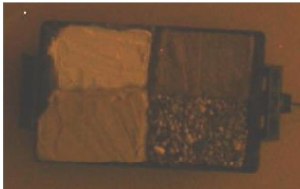
**Figure 3.1:** Image of four different sediments tested (starting from top left, clockwise): Kaolinite, Coarse Sand, Gravel, and Fine Sand.
