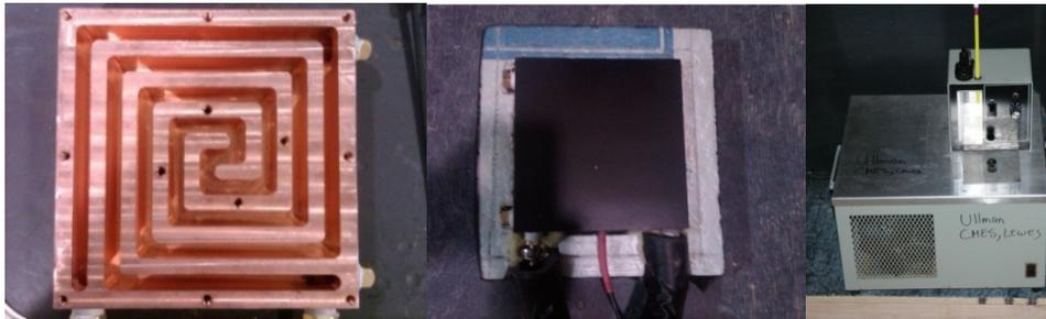
**Figure 2.14:** TRE without cover plate (left); TRE covered, painted, and insulated (center); water bath (right).
