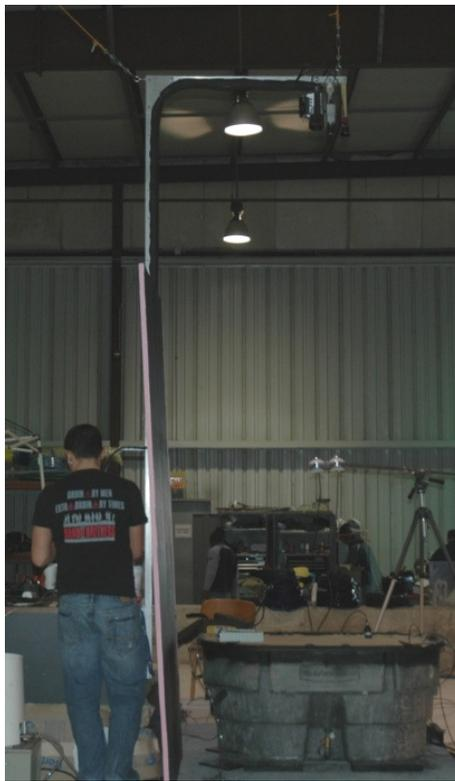
**Figure 2.1:** Overall apparatus set-up with preliminary tank shown and three imagers mounted to secondary goniometer arm.
