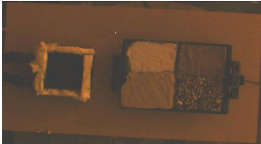
**Figure 2.16:** RGB image of sediment and TRE setup in experiment area. In this image, the hot plate can be seen (right side of image) with all 4 sediments in testing position. The TRE can also be seen to the left of this image. This TRE was insulated to avoid edge effects along the left side of the hot plate.
