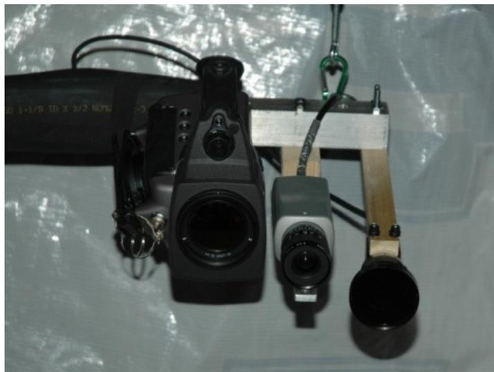
**Figure 2.3:** Imagery mounted to secondary goniometer arm. From left to right: Thermal Imager, RGB Imager, and NIR Imager (discussed in section 2.2).
