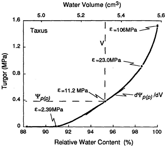
Figure 2.9. The turgor ( $\Psi_{p(p)}$ ) and volume ( $V$ ) of water in the cells of the *Taxus* branch shown in Fig. 2.8. The slope  $d\Psi_{p(p)}/dV$  was measured at each  $\Psi_{p(p)}$  and  $V$ , and the elastic modulus ( $\epsilon$ ) also was calculated. In the example shown, the slope is drawn through a point and  $\epsilon = (0.380 \text{ MPa}/0.180 \text{ cm}^3) \cdot 5.32 \text{ cm}^3 = 11.2 \text{ MPa}$ . Data from J. S. Boyer (unpublished).
