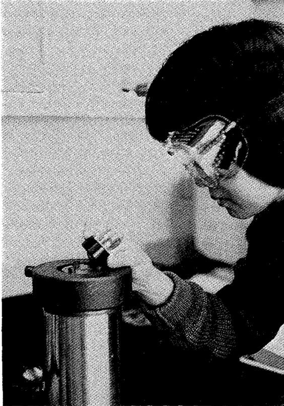
**Figure 2.6.** Measuring the xylem tension with a pressure chamber. Note that the observer always stays to the side of the apparatus and wears safety glasses in case tissue is blown out of the chamber.
