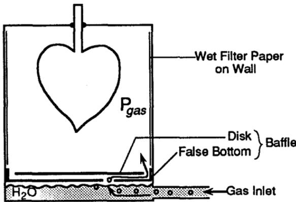
**Figure 2.5.** Water in the bottom of a pressure chamber reduces overheating of the entering gas and humidifies the air around the leaf. A two-part baffle prevents splashing on the leaf. Normally, the chamber wall is also lined with wet filter paper.
