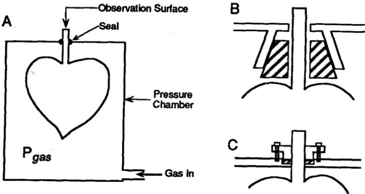
**Figure 2.1.** Pressure chamber design. A) Basic layout of chamber and tissue during pressurization. B) Enlarged view of a seal that is tightened by gas pressure; the seal around the tissue becomes tighter as pressure drives the rubber stopper (cross-hatched) deeper into the cone below the chamber top. C) Enlarged view of a seal that is tightened manually; tightening the screws forces the rubber seal against the tissue.
