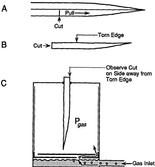
**Figure 2.7.** Sampling a wide grass leaf. Cut across the leaf almost to the midvein (A), tear the leaf toward the apex from the cut (B), and insert the sample in the pressure chamber (C). Observe the appearance of the xylem solution at the cut surface during pressurization but ignore solution appearing close to the torn edge.
