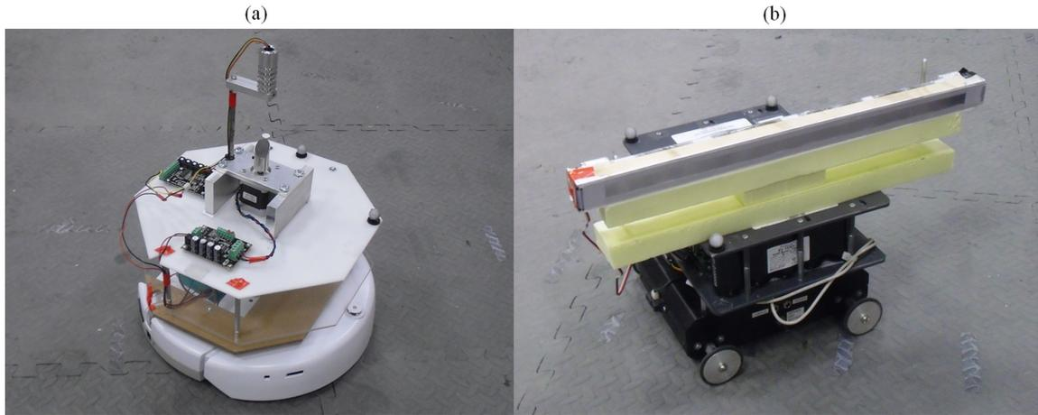
**Figure 4.8:** (a) laser device mounted on the iCreate<sup>TM</sup>; (b) light sensor mounted on the Corobot<sup>TM</sup>
