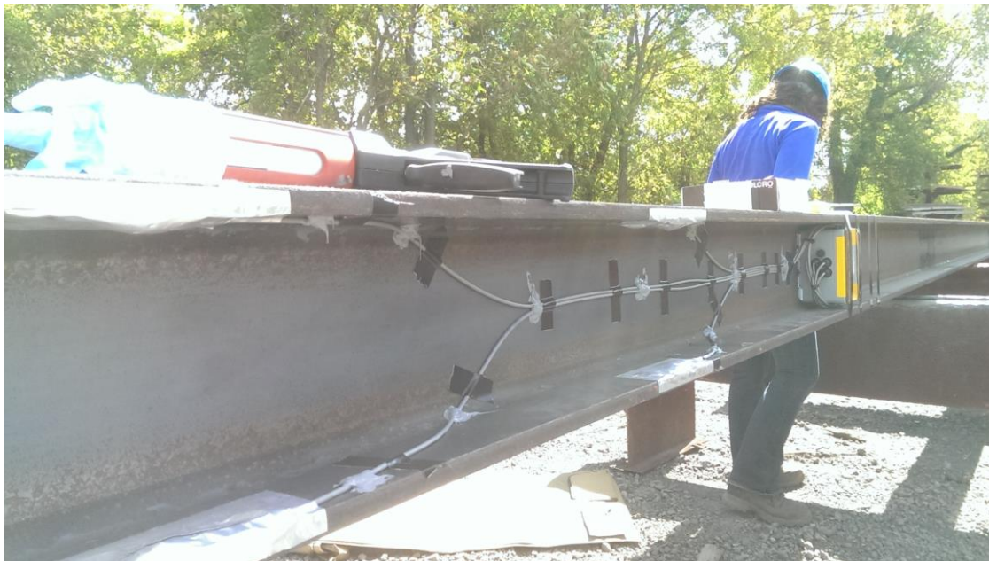
Figure 16: Instrumenting member 3C3 at RCF with weldable strain gauges and WSN nodes
