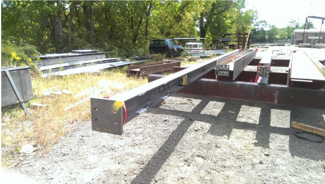
Figure 17: Final instrumentation of the steel members for Purnell Hall
