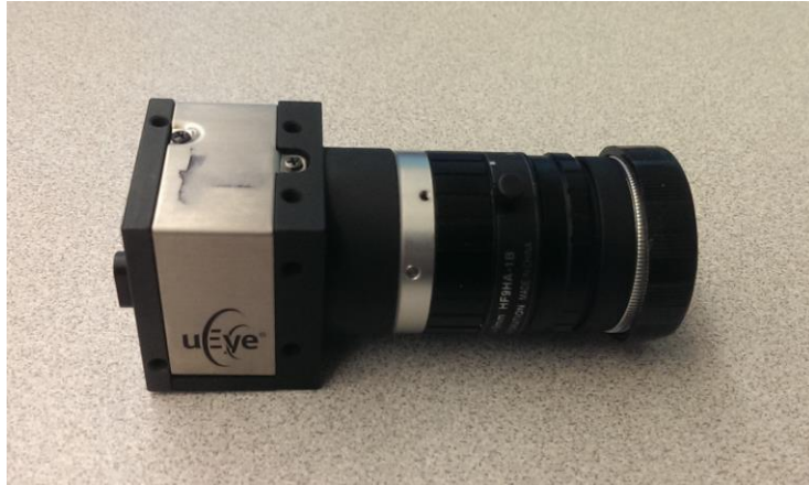
Figure 19: IDS Camera model UI-1540SE that was used for video documentation of the construction site
