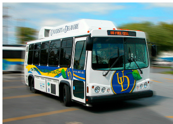
Figure 1. The University of Delaware's 22-foot, 22-seat transit bus equipped with a fuel cell/battery series-hybrid powertrain, manufactured by EBus, Inc. of Downey, CA, USA.
