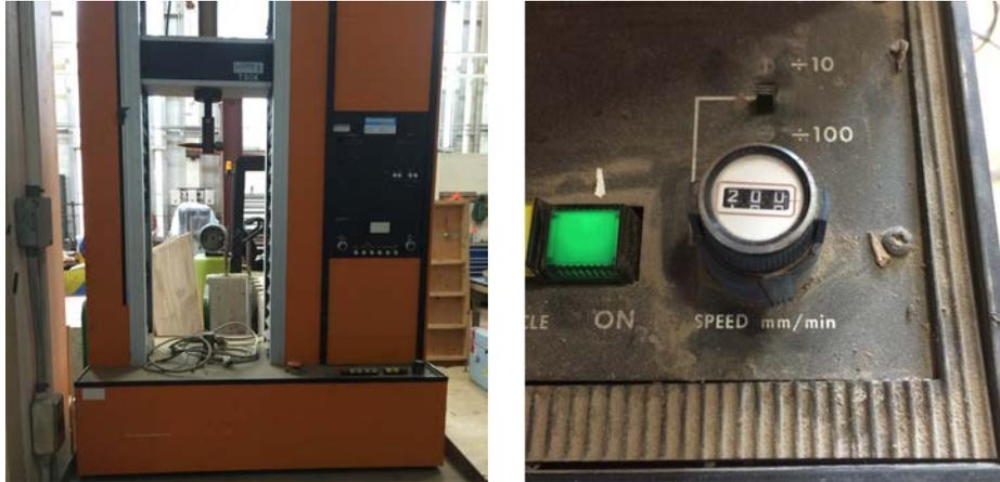
Figure 3.4 The Lloyd T50K Testing Machine (left); Crosshead Speed Dial (right)
