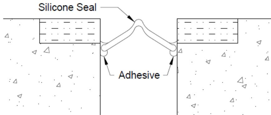
Figure 1.1 Typical SMEJ Cross Section (Preformed Silicone)
