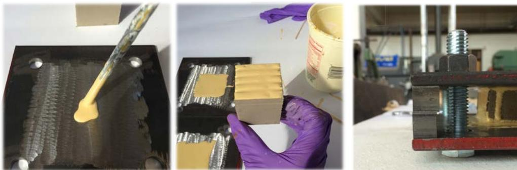
Figure 3.2 Applying Epoxy to Steel (left); Epoxy Applied to Grooved Foam (center); Compressed Plates with Loaded Foam Specimen (right)
