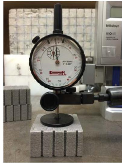
Figure 2.3 Mounting Station and Dial Gauge, Corner Thickness (left); Center Thickness (right)
