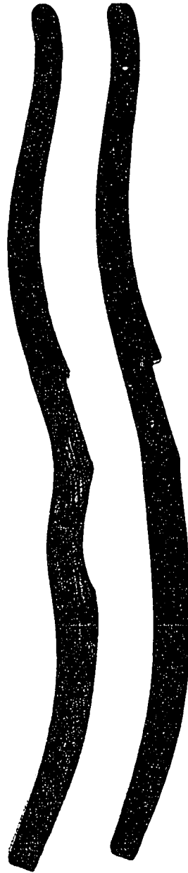
Figure 5.42 Two patterns for rocker stiles from the Kersh shop showing difference in definition of curve. Kersh collection, MAFC.
