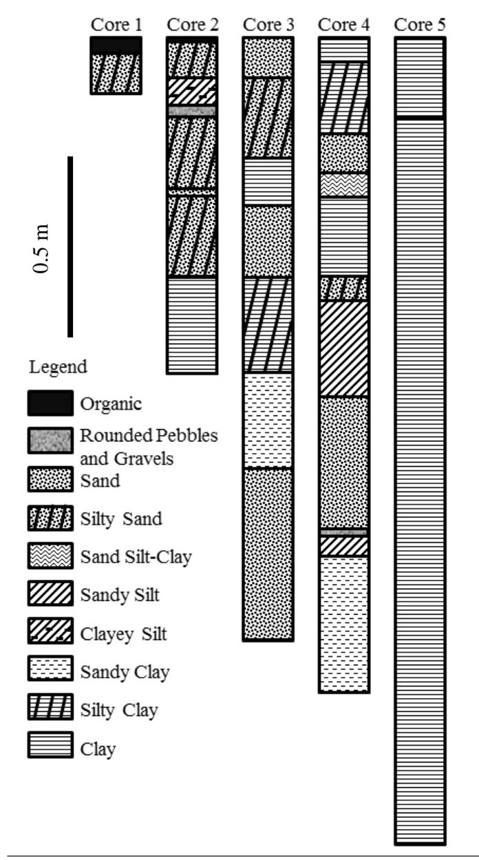
Figure 9: Logs of bucket auger cores collected adjacent to the active channel. Cores displayed in progression from upstream to downstream but do not overlap stratigraphically.
