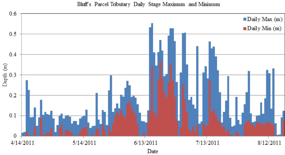
Figure 7: Water stage calculated from onsite HOBO pressure transducer data.
