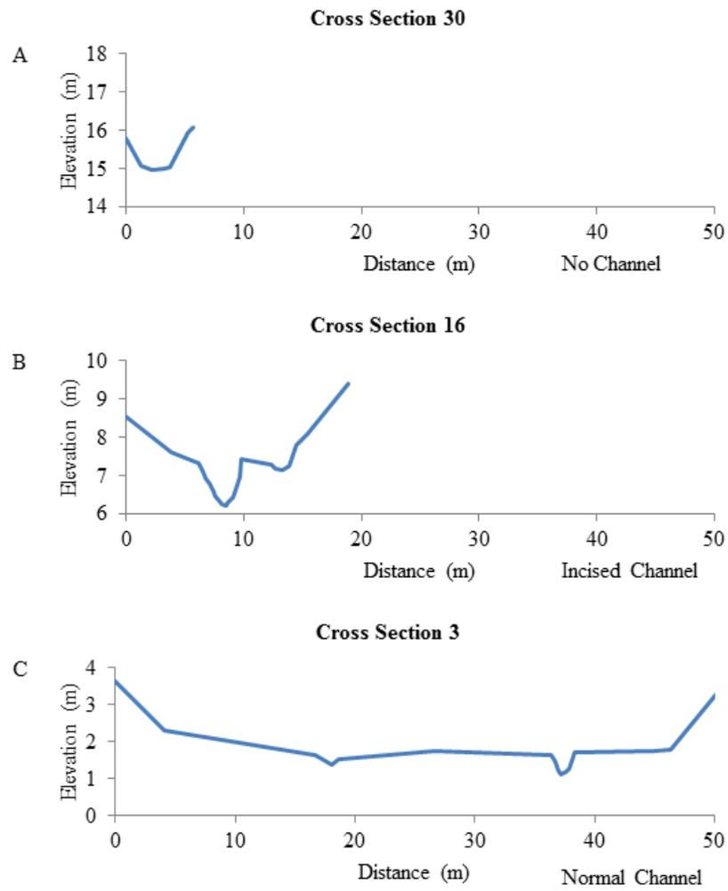
Figure 5: Cross section evolution upstream (A) to downstream (C).
