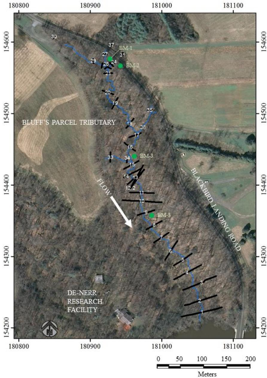
Figure 2: Benchmark locations (green) and valley cross section location, orientation, and extent (black) (2010 Orthoimage courtesy of United States Geological Survey).
