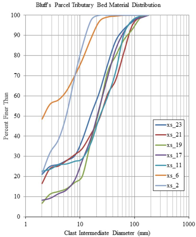
Figure 6: Grain size distributions for the bed material of Bluff's Parcel Tributary. Location indicated by cross section ID, ID numbers decrease in the downstream direction. Distributions fine downstream.
