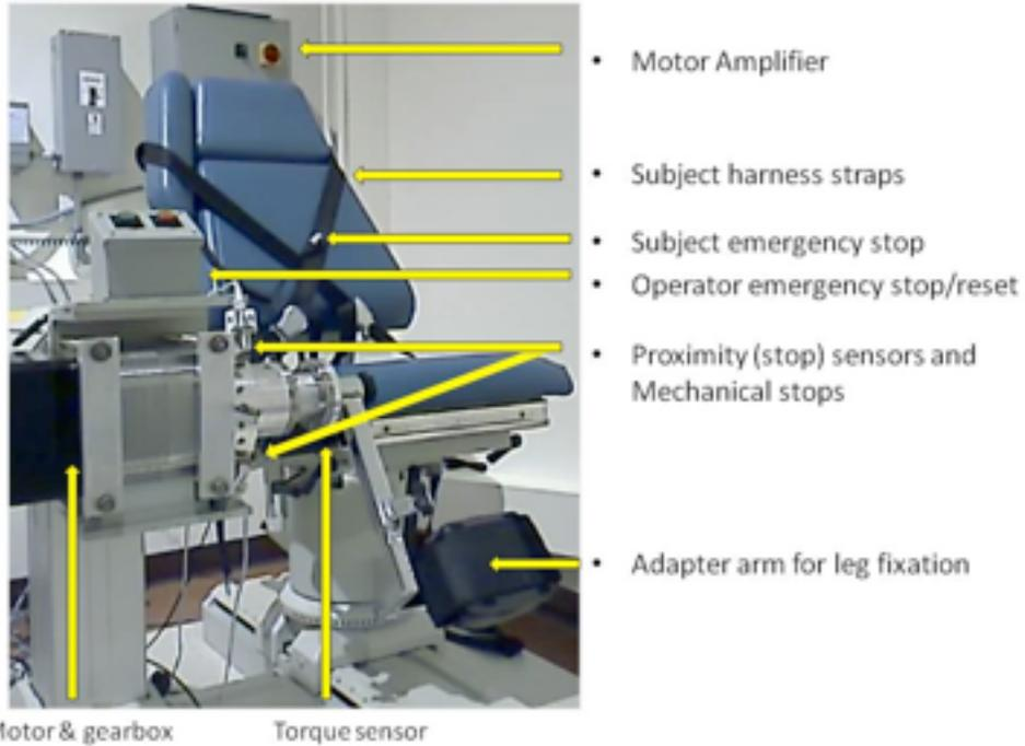
Figure 1. Stiffness and Proprioception Assessment Device (SPAD)
