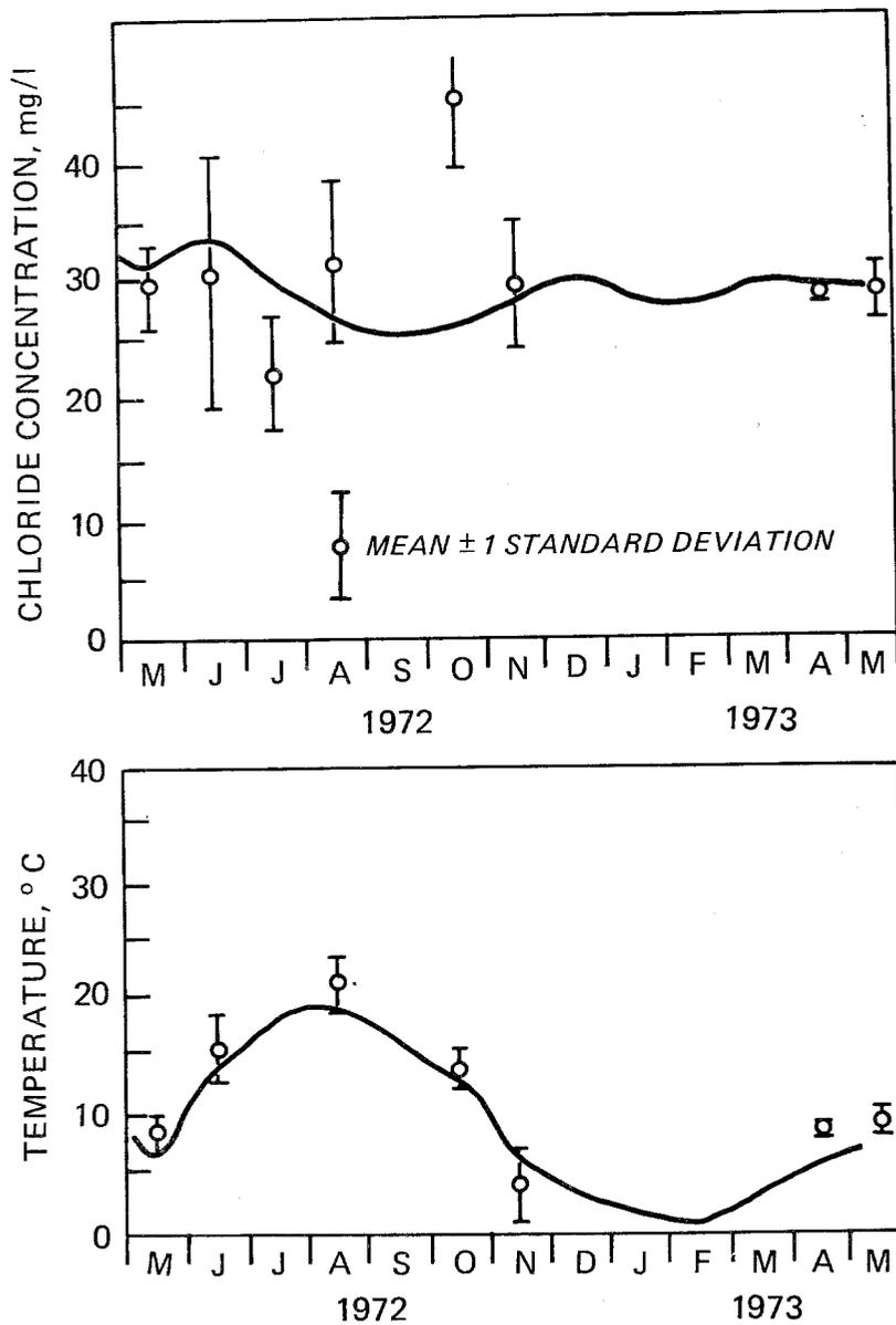
Figure 68 Typical calibration of advective and dispersive regime, chloride and temperature, segment 21.
