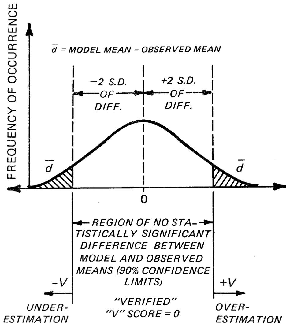
Figure 11 Determination of verification score, V
