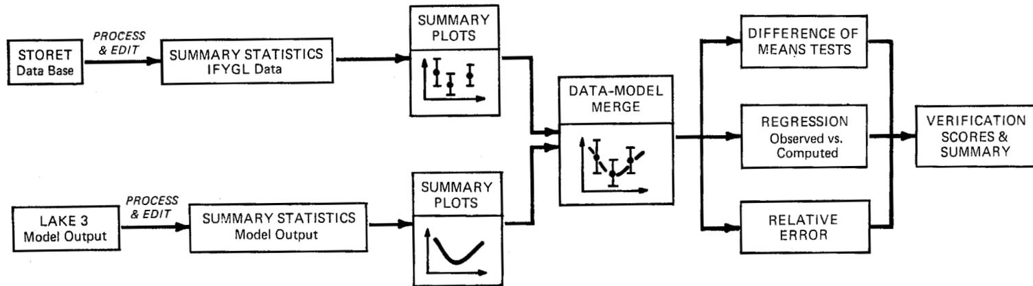
Figure 4 Flow diagram for model verification analysis
