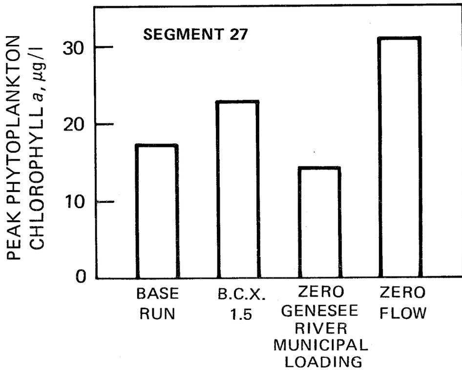
Figure 78 Comparison of calculated peak phytoplankton embayment concentrations under different conditions on nutrient inputs and transport.
