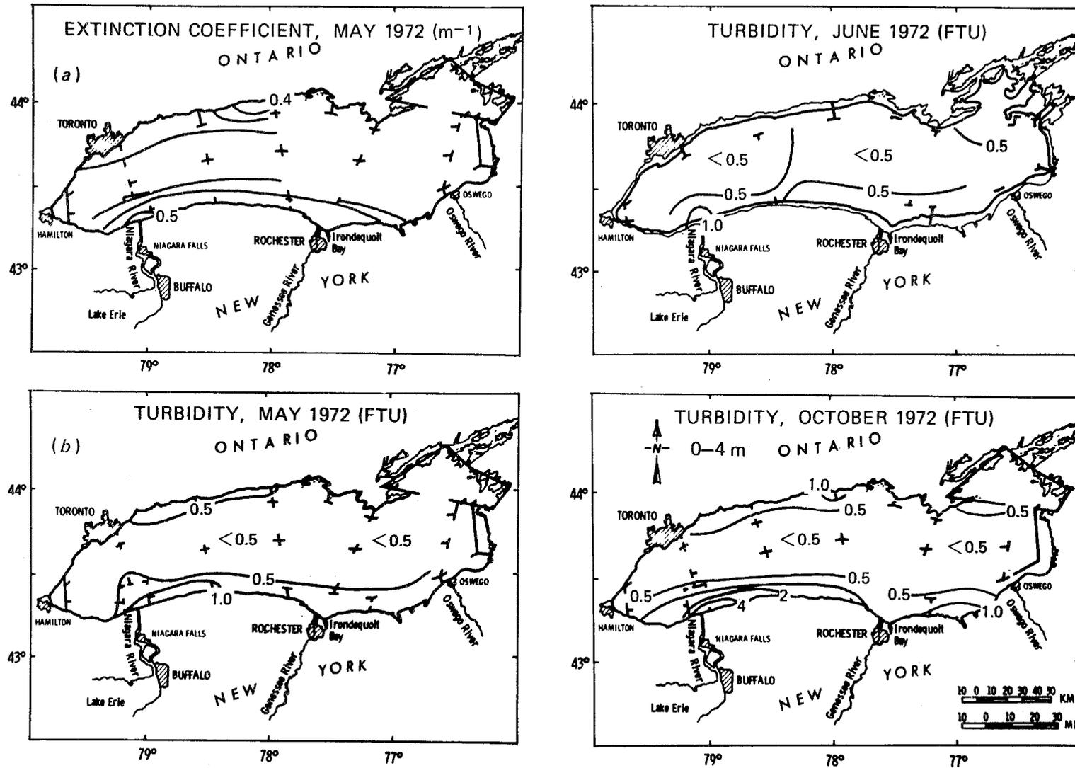
Figure 20 Variation of (a) extinction coefficient (EPA-CCIW data) and (b) turbidity (CCIW data) for selected months, 0-4 m.
