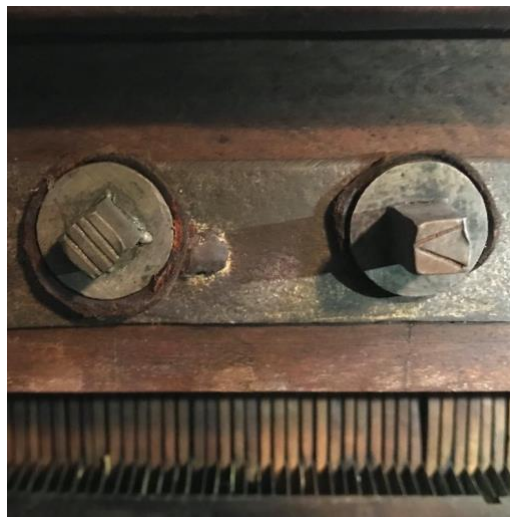
Figure 18 Roman numerals are also present on the metal bolts that keep the front needle plates in place on Miller's frame. Knitting frame. Textile & Costume Collection, Thomas Jefferson University. Courtesy of the Textile & Costume Collection, Thomas Jefferson University.
