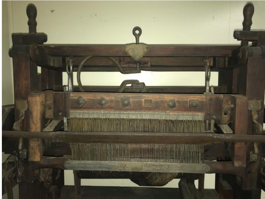
Figure 14 The carcass of Godfrey Miller's knitting frame, which is made up of the jacks, jack sinkers, bearded needles, and presser bar. Knitting frame. Textile & Costume Collection, Thomas Jefferson University. Courtesy of the Textile & Costume Collection, Thomas Jefferson University. Photo by the author.
