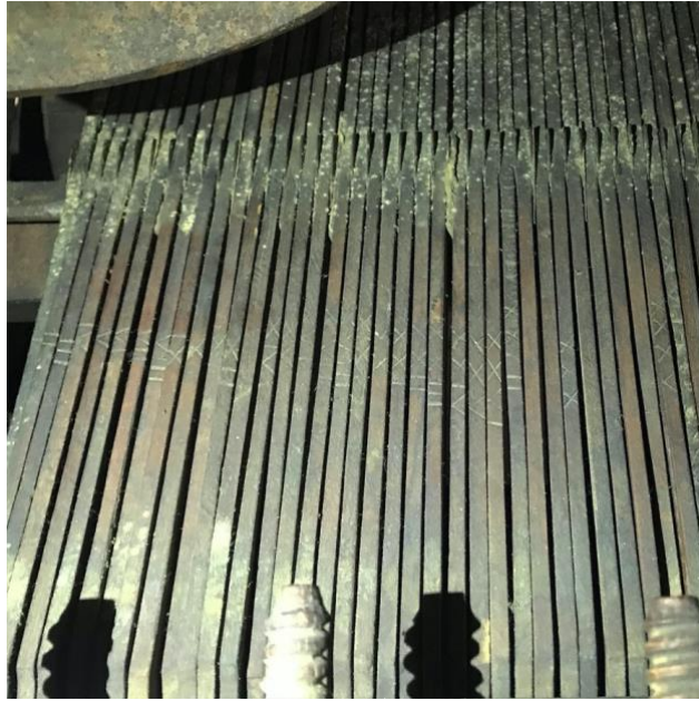
Figure 17 Roman numerals are carved into the original wooden jacks of Miller's frame, while the replacement jacks are blank. Knitting frame. Textile & Costume Collection, Thomas Jefferson University. Courtesy of the Textile & Costume Collection, Thomas Jefferson University.
