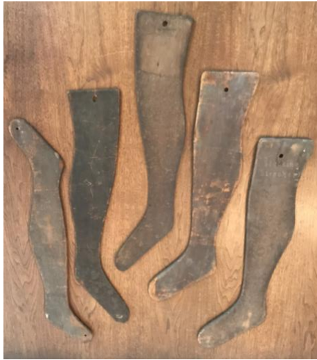
Figure 25 Nineteenth-century stocking boards, also called “stocking boards” used by Germantown knitting mills to block stockings into shape. Stocking boards. Germantown Historical Society. Courtesy of Germantown Historical Society/Historic Germantown. Photo by the author.
