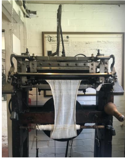
Figure 12 A late eighteenth-century knitting frame made in England. Notable construction differences between this frame and Godfrey Miller's frame are mentioned in the Appendices. Knitting Frame. Framework Knitters Museum. Courtesy of Framework Knitters Museum. Photo by the author.
