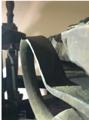
Figure 15 The main spring on Miller's frame had to be fit inside the crossbeam, shown by the gouge marks in the wood. Knitting frame. Textile & Costume Collection, Thomas Jefferson University. Courtesy of the Textile & Costume Collection, Thomas Jefferson University.
