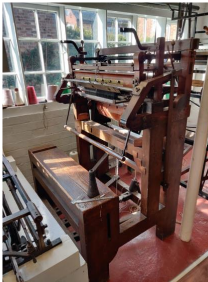
Figure 13 Eighteenth-century knitting frame used in Germany, also called a "Saxon" frame. Saxon Frame. Framework Knitter's Museum. Courtesy of the Framework Knitter's Museum. Photo by the author.
