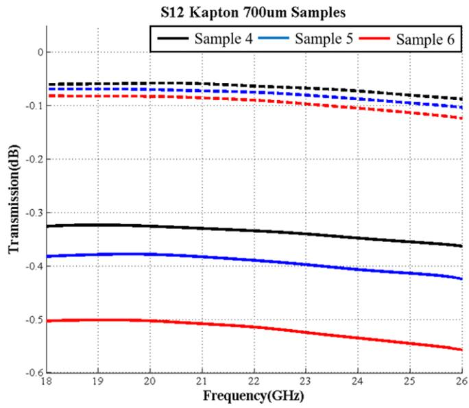
Figure 4.8 Kapton nScript printed 700μm samples. The solid lines represent the ninety degree orientation and the dashed lines represents the zero degree orientation. The shift from samples is due to the amount material deposited. This corresponds well with the measurements in Table 4.1.
