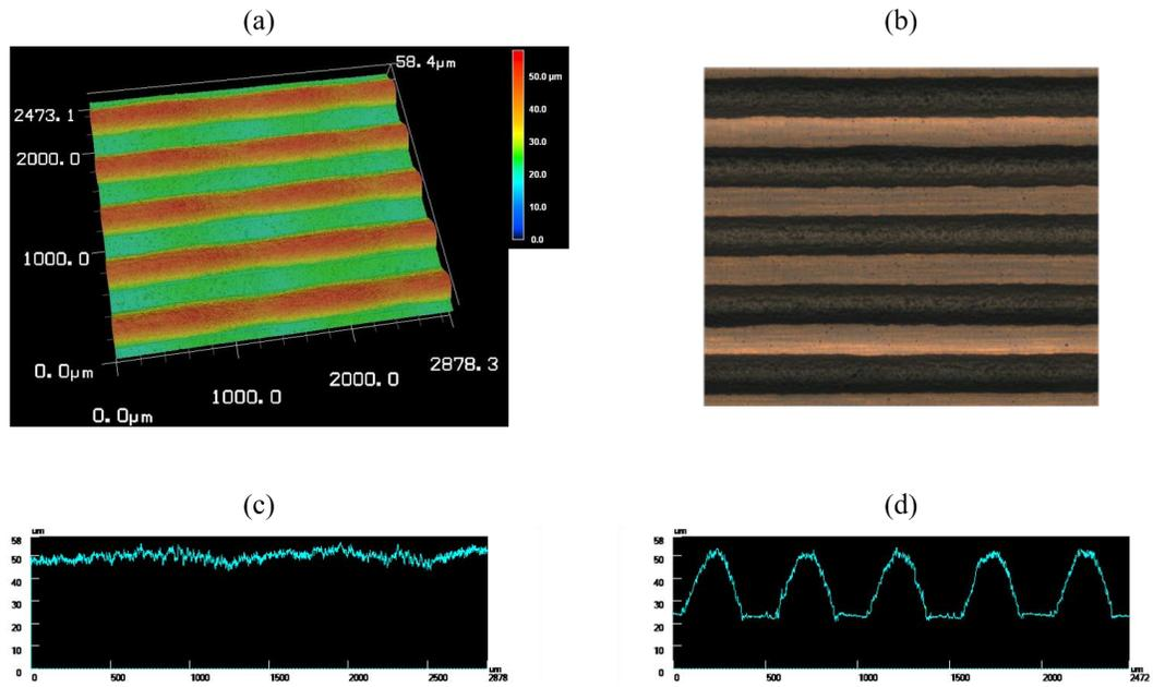
Figure 4.4 Confocal imaging of 500µm period nScript printed Kapton sample: (a) 3-D profile of sample; (b) optical image of sample; (c) horizontal profile of line; (d) profile of line width.
