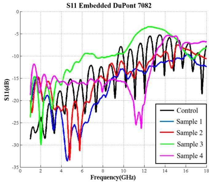
Figure 4.11 S11 plot for nScript printed transmission line samples with DuPont 7082 embedded within the substrate.
