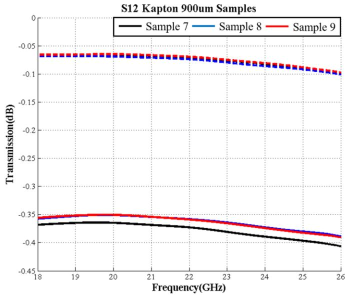
Figure 4.9 Kapton nScript printed 900μm samples. The solid lines represent the ninety degree orientation and the dashed lines represents the zero degree orientation. The zero and ninety degree orientations of these samples were very closely matched with one another. The minor shift from samples is due to the amount material deposited. This corresponds well with the measurements in Table 4.1.
