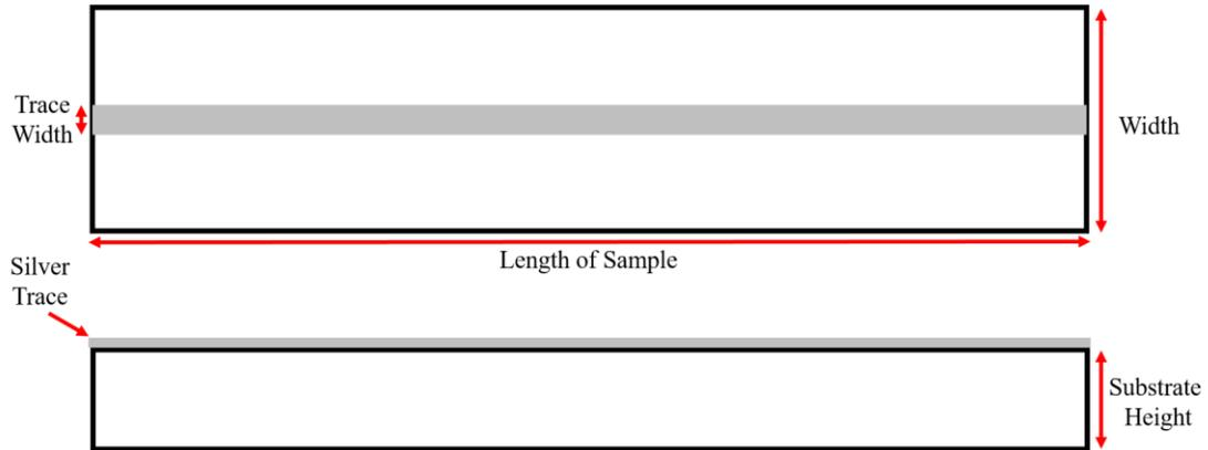
Figure 3.7 Baseline transmission line of polycarbonate, top view (top) and side view (bottom).
