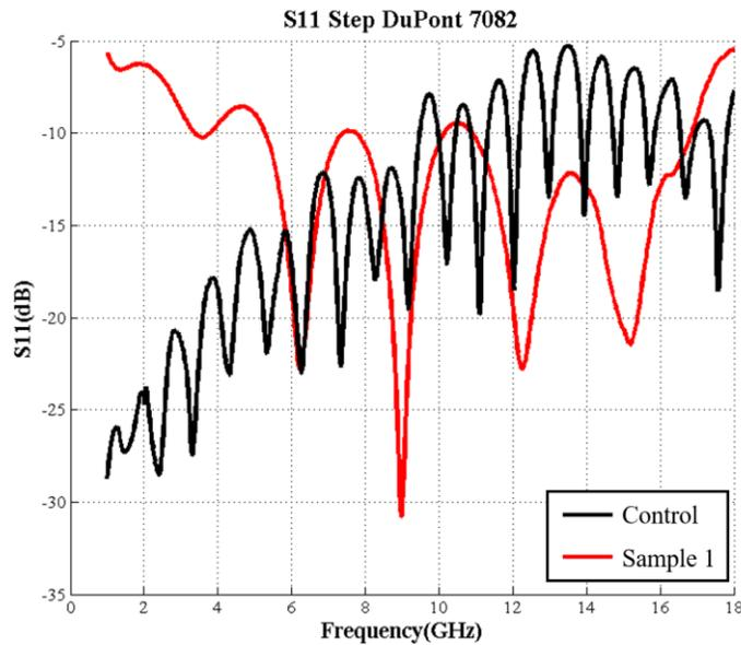
Figure 4.15 S11 plot for nScript printed transmission line sample with DuPont 7082 steps printed at the surface of the substrate.
