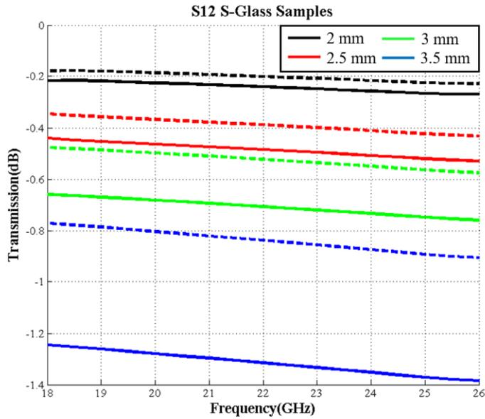
Figure 4.5 S-glass screen printed samples. The solid lines represent the ninety degree orientation and the dashed lines represents the zero degree orientation.
