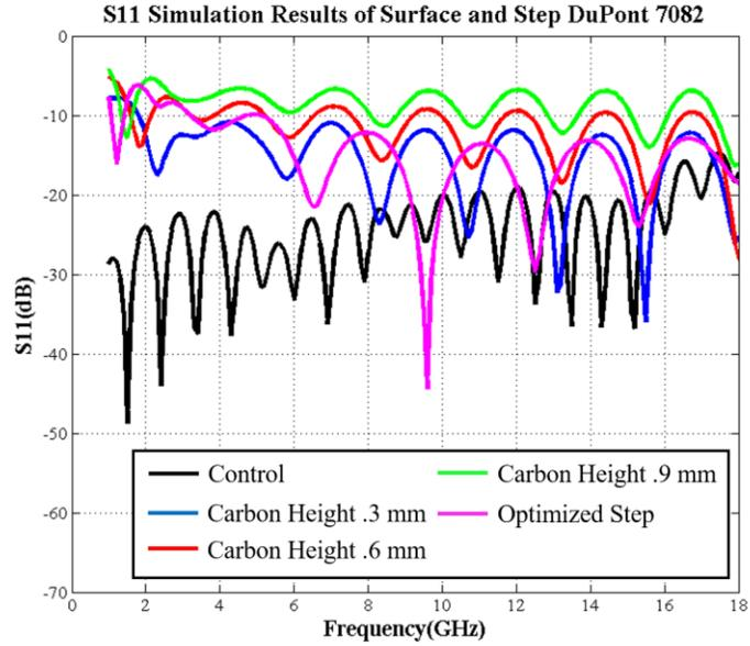
Figure 5.8 S11 plot of simulated transmission line samples with DuPont 7082 slab located at the surface of the substrate and optimized step.
