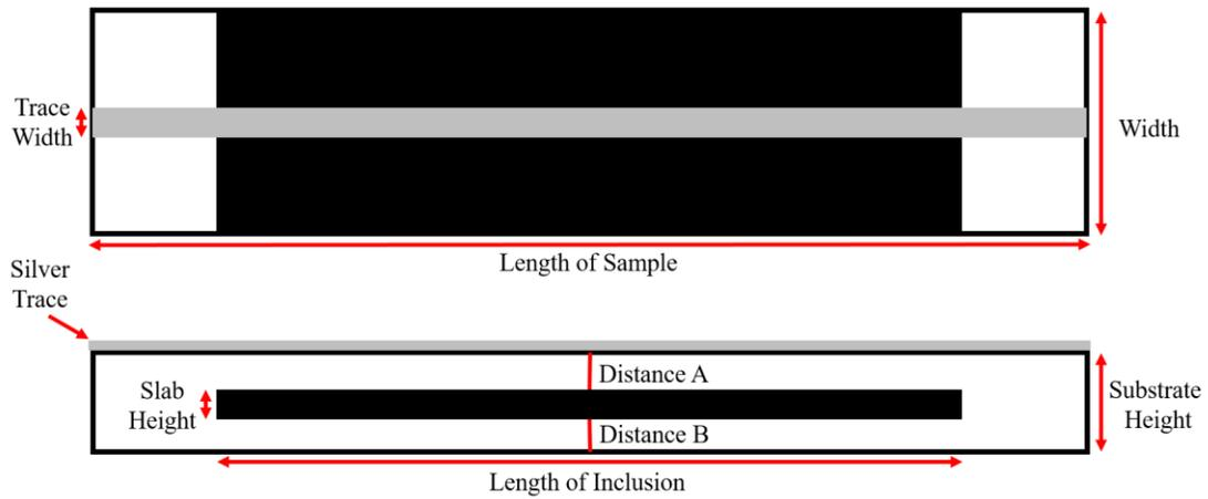
Figure 3.8 Transmission line with DuPont 7082 slab centered, top view (top) and side view (bottom).
