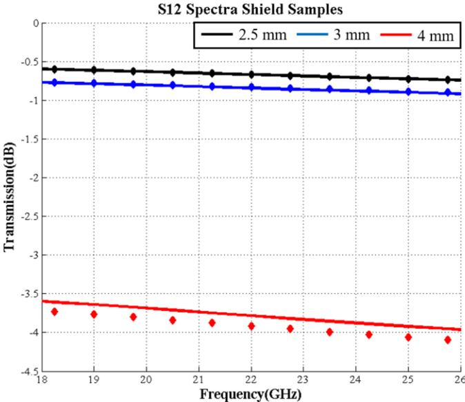
Figure 4.6 Spectra shield screen printed samples. The solid lines represent the ninety degree orientation and the diamond lines represents the zero degree orientation.
