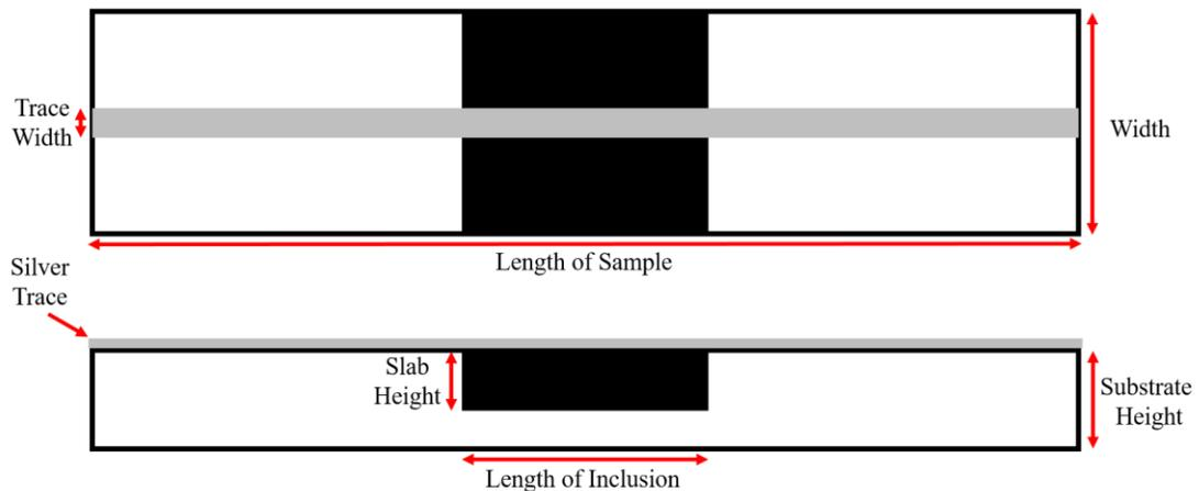
Figure 3.9 Transmission line with DuPont 7082 slab at top of substrate, top view (top) and side view (bottom).
