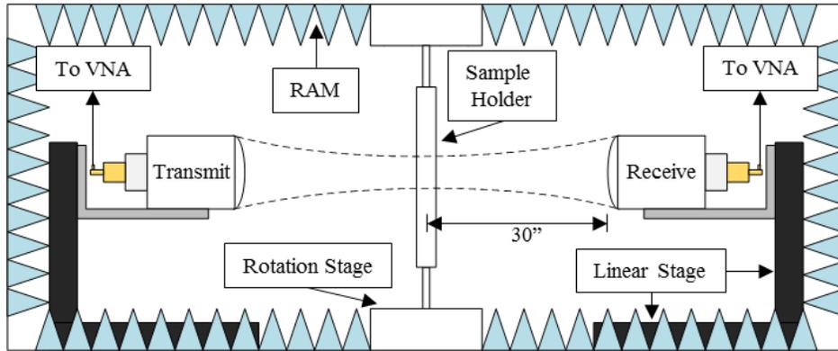
Figure 4.1 Focused beam measurement system within a radar absorbing anechoic chamber.
