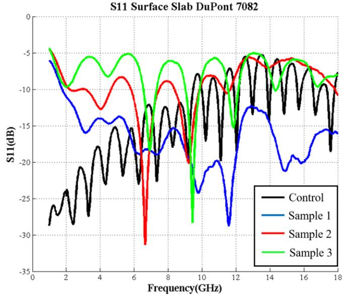
Figure 4.13 S11 plot for nScript printed transmission line samples with DuPont 7082 slab printed at the surface of the substrate.
