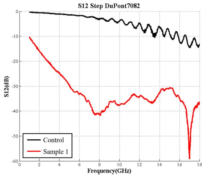
Figure 4.14 S12 plot for nScript printed transmission line sample with DuPont 7082 steps printed at the surface of the substrate.
