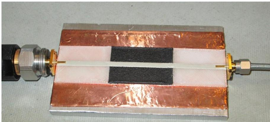
Figure 4.2 Transmission line fixture connected to VNA to measure S parameters.
