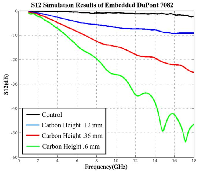
Figure 5.3 S12 plot of simulated transmission line samples with DuPont 7082 slab embedded within the substrate. The carbon height is the thickness of the carbon that is centered within a 1.2 mm thick substrate.
