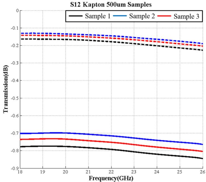
Figure 4.7 Kapton nScript printed 500 $\mu\text{m}$  samples. The solid lines represent the ninety degree orientation and the dashed lines represents the zero degree orientation. The shift from samples is due to the amount material deposited. This corresponds well with the measurements in Table 4.1.
