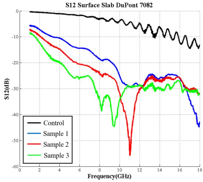
Figure 4.12 S12 plot for nScript printed transmission line samples with DuPont 7082 slab printed at the surface of the substrate.
