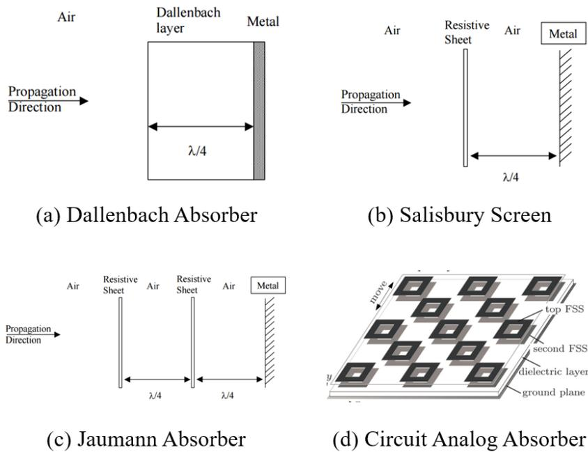
Figure 1.1 Illustration of various common methods to design resonant EM absorbers.
