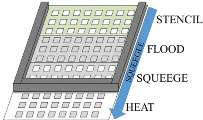
Figure 3.1 Flow of screen printing process
