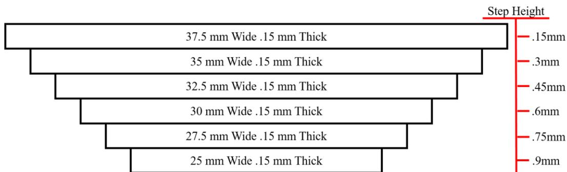
Figure 3.11 Step profile of DuPont 7082 within polycarbonate.
