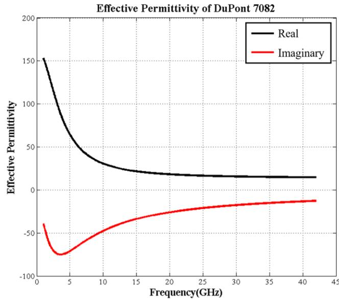
Figure 5.1 Effective permittivity of DuPont 7082 based on rigorous coupled wave analysis and the Debye equation.
