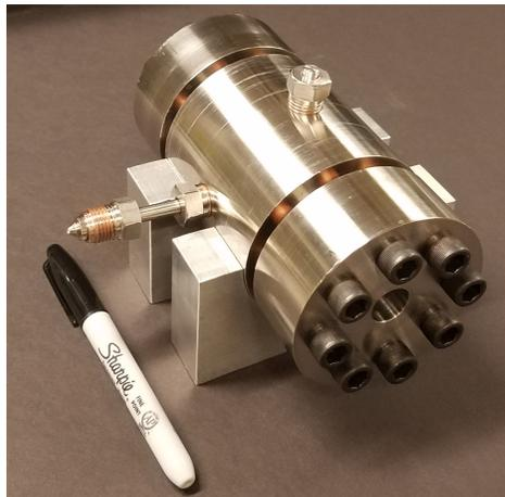
**Figure 2.5:** Assembled high-pressure cell resting in aluminum jaws. Side left connection goes to sample gauge and piston. Top port is shown with plug.
