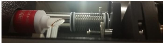
**Figure A.5:** Image of rear Brewster window facing downwards. This window is cleaned from bottom to top.
