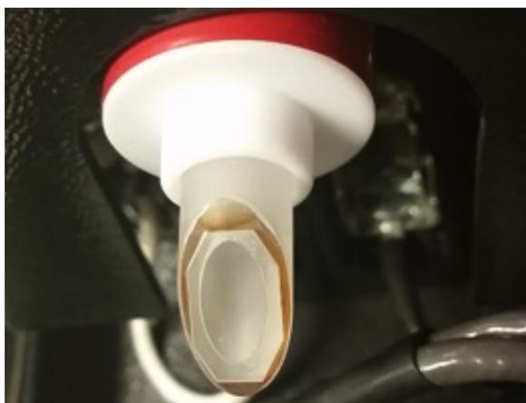
**Figure A.6:** Front Brewster window face before cleaning by the “Hemostat and Lens Tissue Method”.
