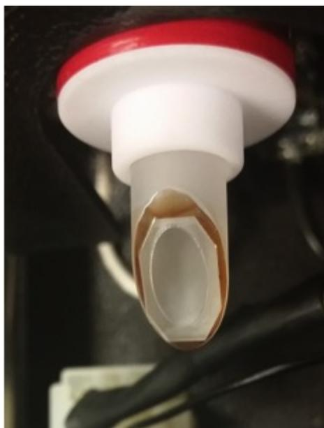
**Figure A.7:** Front Brewster window face after cleaning by the “Hemostat and Lens Tissue Method”.
