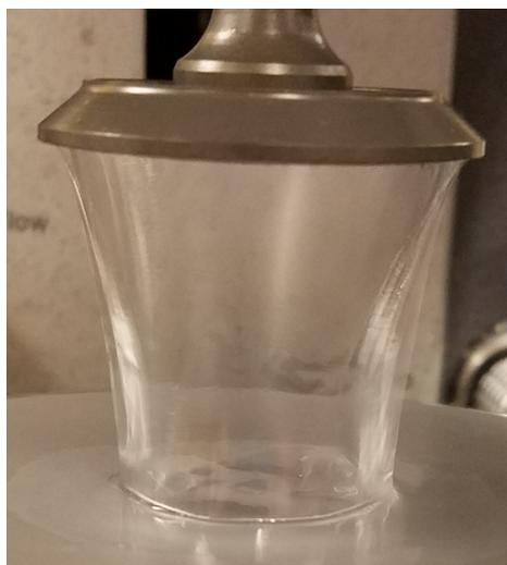
**Figure 4.6:** Image of 0.3 wt% guar gum with 40 ppm boron. Geometry shown is a 40 mm 4° cone and peltier plate.
