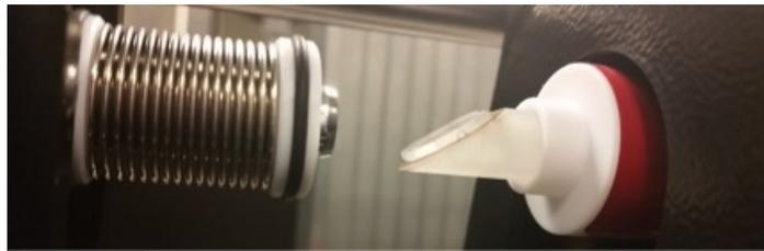
**Figure A.4:** Image of front Brewster window facing upwards. This window is cleaned from top to bottom.
