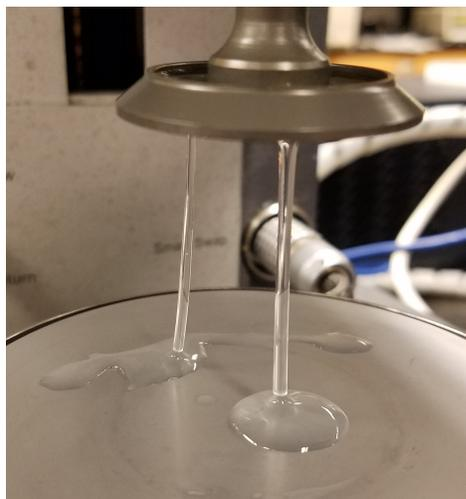
**Figure 4.5:** Image of 0.3 wt% guar gum with 60 ppm boron. Geometry shown is a 40 mm 4° cone and peltier plate.
