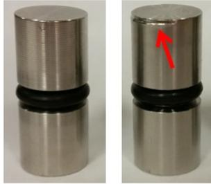
**Figure 2.6:** Piston with (right) and without deformation (left) caused by bottoming out.
