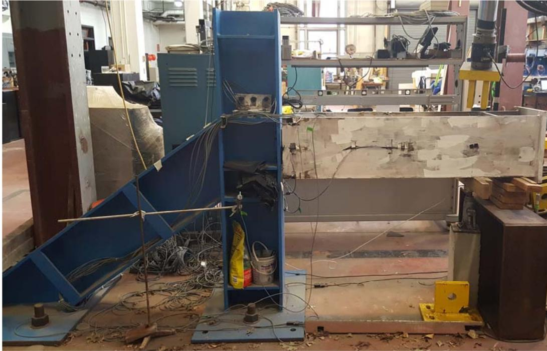
Figure 5.17: South view of the laboratory test setup, weak axis bending configuration
