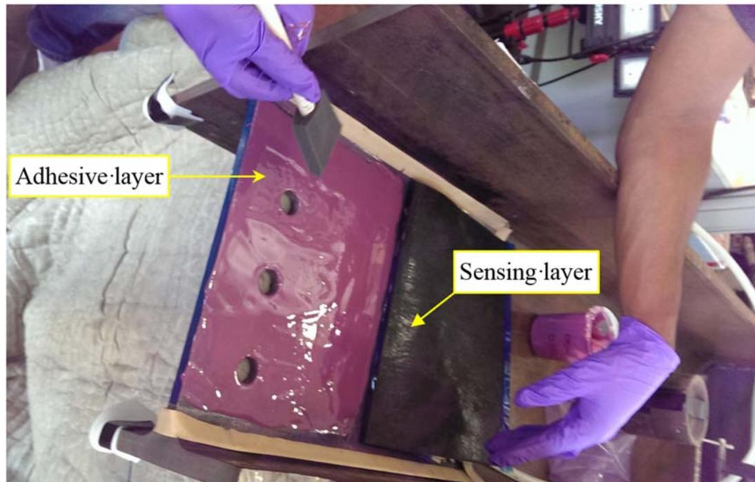
Figure 5.11: Adhesive layer application to install the sensing skin
