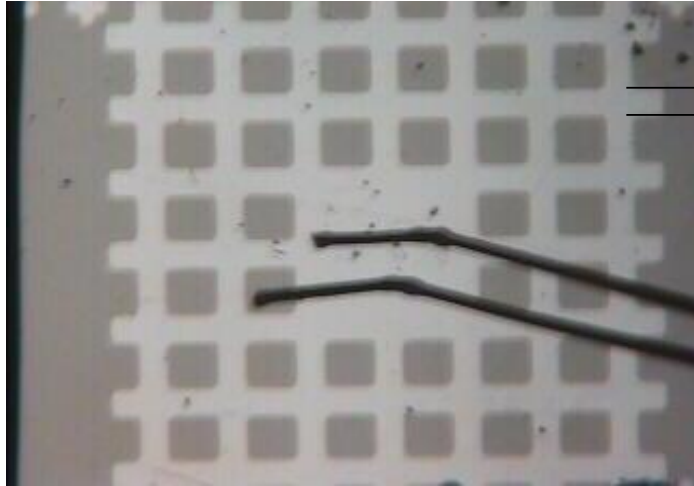
Figure 3.6: Top view of the device showing the Al meshes with two Au wire bonded
