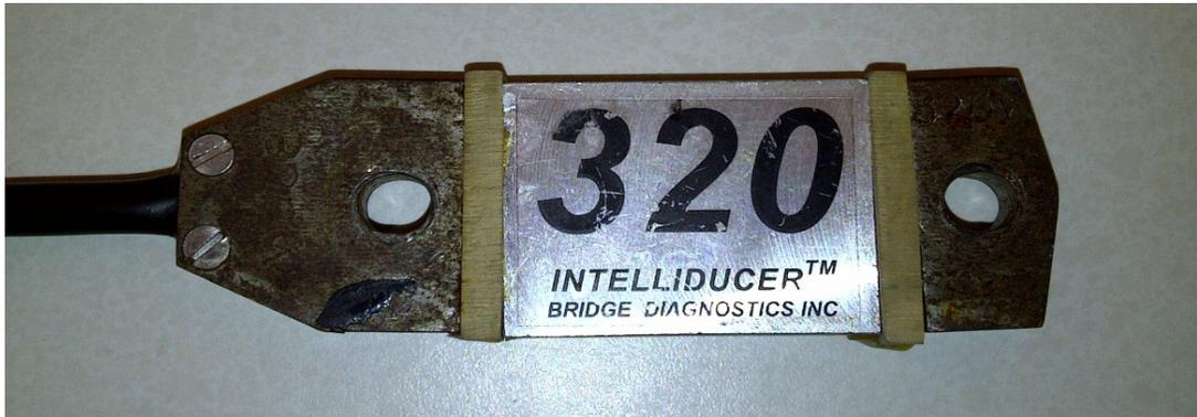
**Figure 3.2** BDI strain transducer ST-350.
