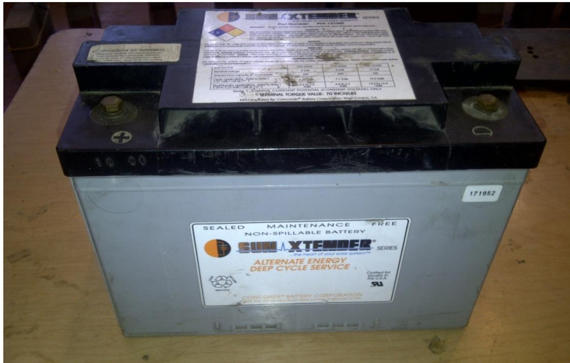
**Figure 3.7** One of two 12V batteries used to power the monitoring system.
