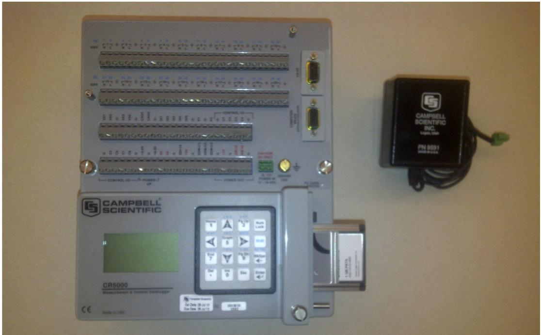
**Figure 3.1 CR5000 data logger with 120VAC adapter and PCMCIA data card.**
