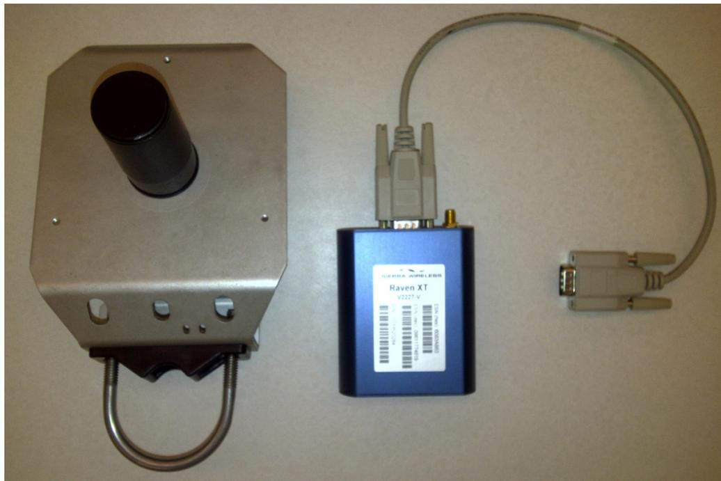
**Figure 3.5 Raven XTV cellular modem and Omni Directional Antenna**
