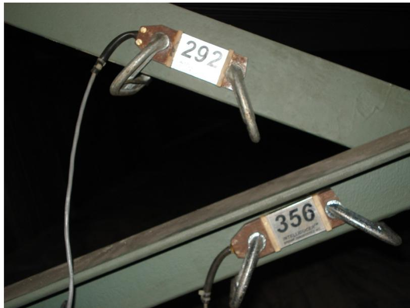
**Figure 3.12** BDI transducers clamped to the bolted legs of cross frame angles.
