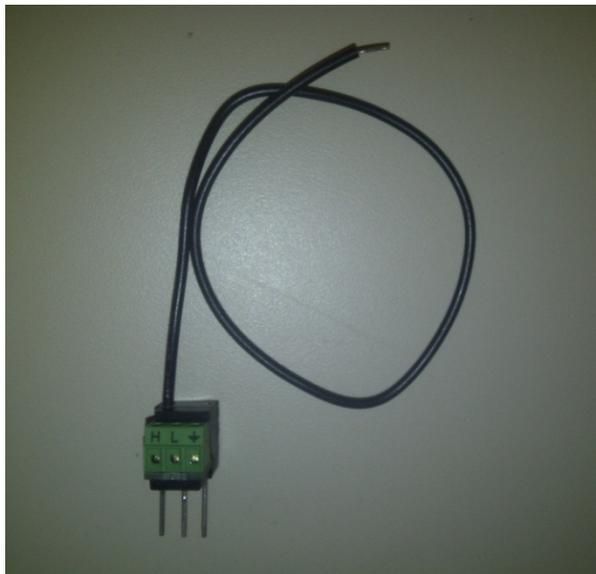
**Figure 3.4** Campbell Scientific Terminal Input Modules to be used with foil gages/
