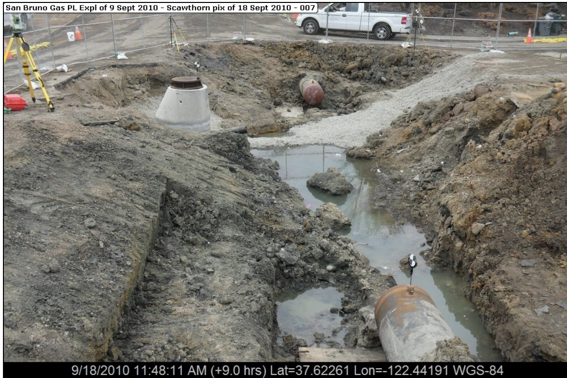
Figure 2 Gas explosion crater (C. Scawthorn)
