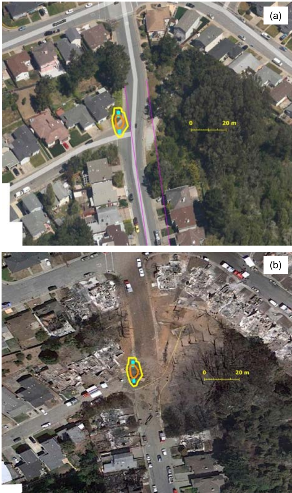
Figure 6 Site (a) before and (b) after explosion with crater's approximate upper (yellow) and lower (orange) outline
