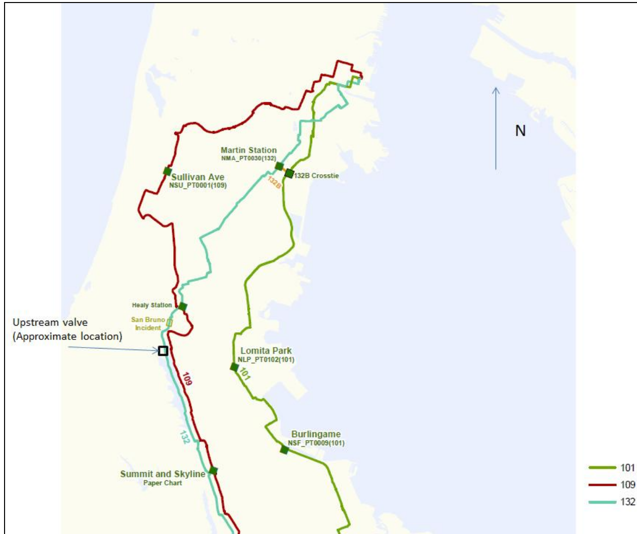
Figure 25 Schematic of pressure points LT system (NTSB 2011f)
