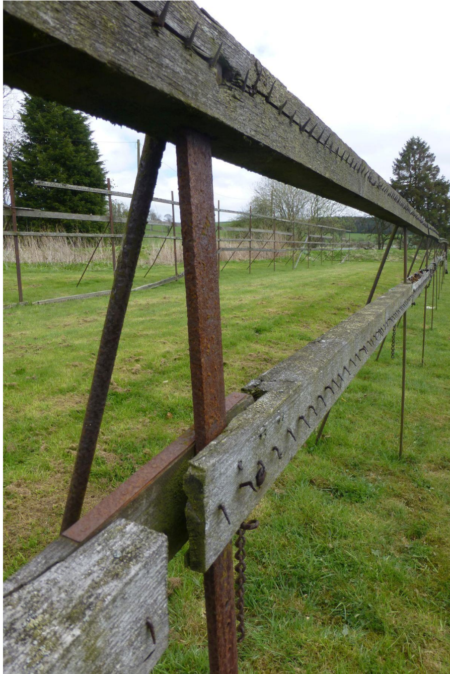
Figure 26 Tenter hooks on a tenter frame at Otterburn Mill. This tenter frame in Otterburn, Northumberland, in the northeast of England, date to the eighteenth-century. The hooks in the wooden beams were used to secure the cloth. The lower beam could be adjusted in height to put tension on the cloth. Photo © Russel Wills (cc-by-sa/2.0). geograph.org.uk/p/5762310
