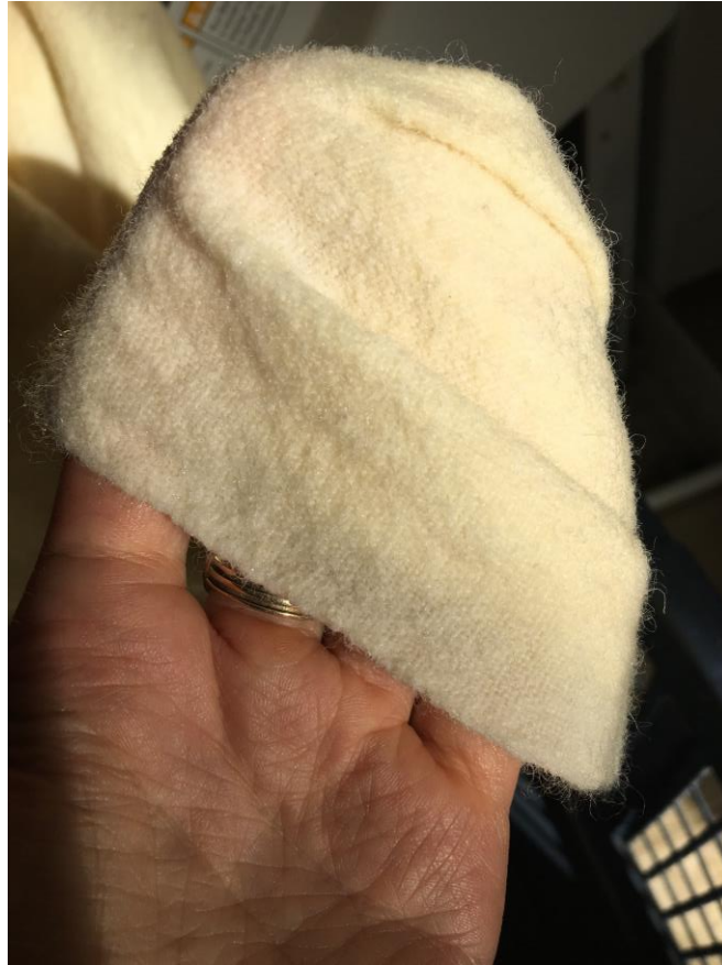
Figure 22 Wet cloth in the process of being fulled. Here the yarns are beginning to come together but are still easily distinguished from each other. Photo by the author.
