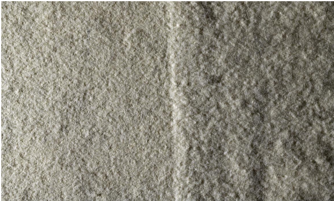
Figure 55 Detail showing the difference between the men's wear flannel before (right) and after pressing (left). The raking light clearly shows that the surface of the pressed cloth is much flatter and smoother than the unpressed cloth. Photo by James Schneck, Winterthur Museum.
