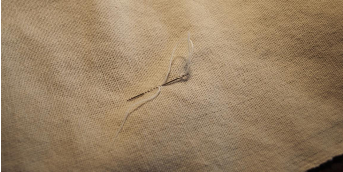
Figure 47 Darning in warp threads which had to be repaired during weaving. This process involved threading the broken yarn ends onto a needle and reweaving them into the cloth for a short distance. Photo by the author.
