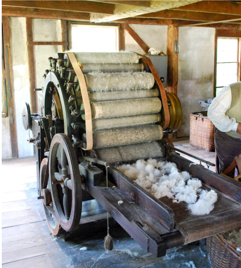
Figure 33 The feed belt and carding cylinders of one of Old Sturbridge Village's nineteenth-century carding machine. Photo by the author.
