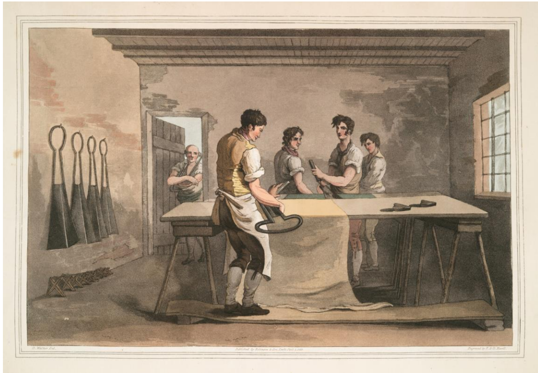
Figure 30 This image depicts cloth shearers at work and shows several sets of cropping shears hanging on the wall. Below the shears sit several napping frames, for smoothing the nap of the cloth between shearings. The Cloth Dresser, The Costume of Yorkshire: illustrated by a series of forty engravings, being fac-similes of original drawings. With descriptions in English and French , (London: Walker, George and R and D Havell, engraver, 1814). From The New York Public Library . This image is in the public domain. https://digitalcollections.nypl.org/items/510d47dc-dc9b-a3d9-e040-e00a18064a99
