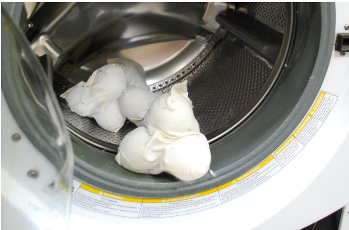
Figure 48 The muslin lacrosse ball “packages” which I used to aid fulling in the washing machine. Photo by the author.
