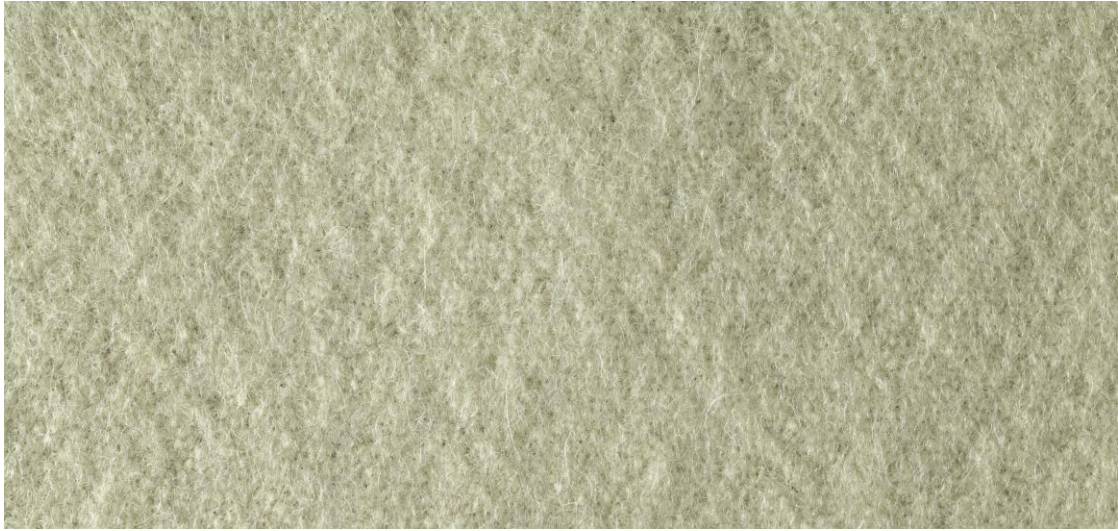
Figure 53 Close-up of “women’s wear flannel” in raking light. The cloth shown here lost fifteen percent of its length in fulling. While it is clearly much fuzzier and more felted than the washed cloth, it is still possible to see some of the woven structure. Photo by James Schneck, Winterthur Museum.
