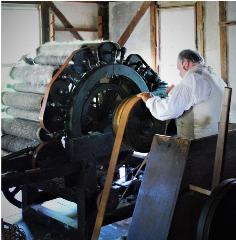
Figure 6 Tom Kelleher, Historian and Curator of Mechanical Arts at Old Sturbridge Village, adjusting the leather drive belt powering one of the museum's nineteenth-century carding machines. Image by the author.
