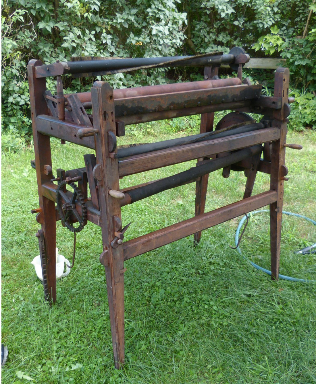
Figure 39 An early nineteenth-century shearing machine, missing its blade, similar in design to Seth Parson's 1819 patent. Courtesy of Peggy Hart. Photo by Jean Hosford
