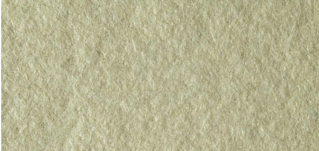
Figure 54 Close-up of “men’s wear flannel” in raking light. The cloth shown here lost twenty-five percent of its length in fulling. This cloth is so heavily fulled that the woven structure is entirely obscured. Photo by James Schneck, Winterthur Museum.
