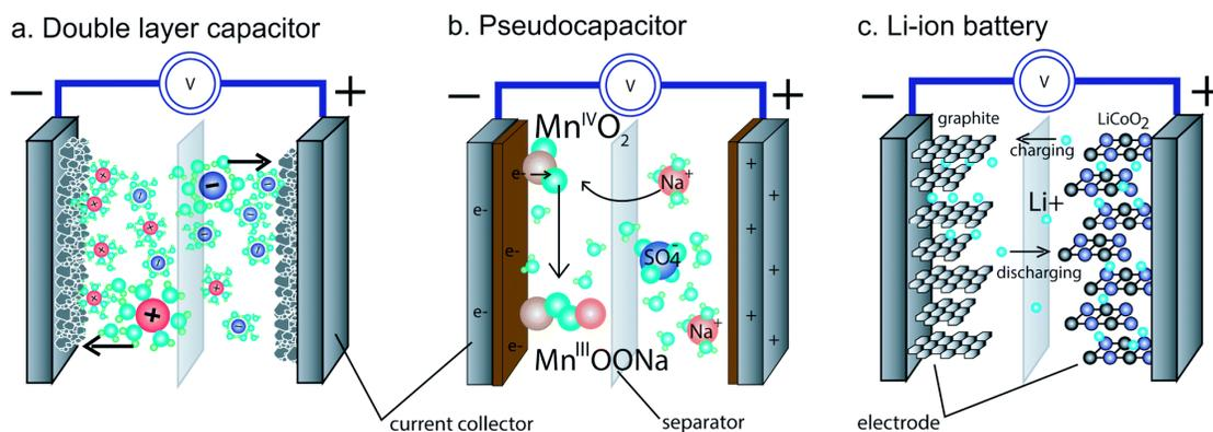
Figure 1.2 Illustrations for an (a) all carbon EDLC, (b) a pseudocapacitor and (c) a lithium-ion battery. All devices have an active material (e.g., carbon, MnO<sub>2</sub>, LiCoO<sub>2</sub>), current collectors, a separator, and an electrolyte, (e.g., Na<sub>2</sub>SO<sub>4</sub>, or LiPF<sub>6</sub> solutions). Reprinted with permission from reference 104 @ 2014, Royal Society of Chemistry
