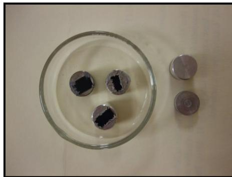
Figure 2.4 Aluminum stubs used for taking SEM images.
