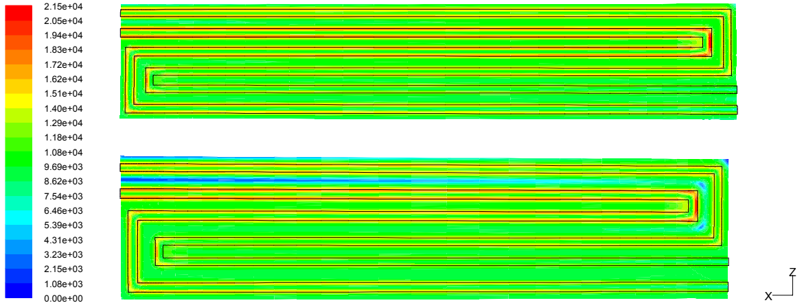
Figure 5.3: Best (top) and worst (bottom) individuals' contour plots of current density ( A/m^2 ) at the cathode GDL-CL interface.
