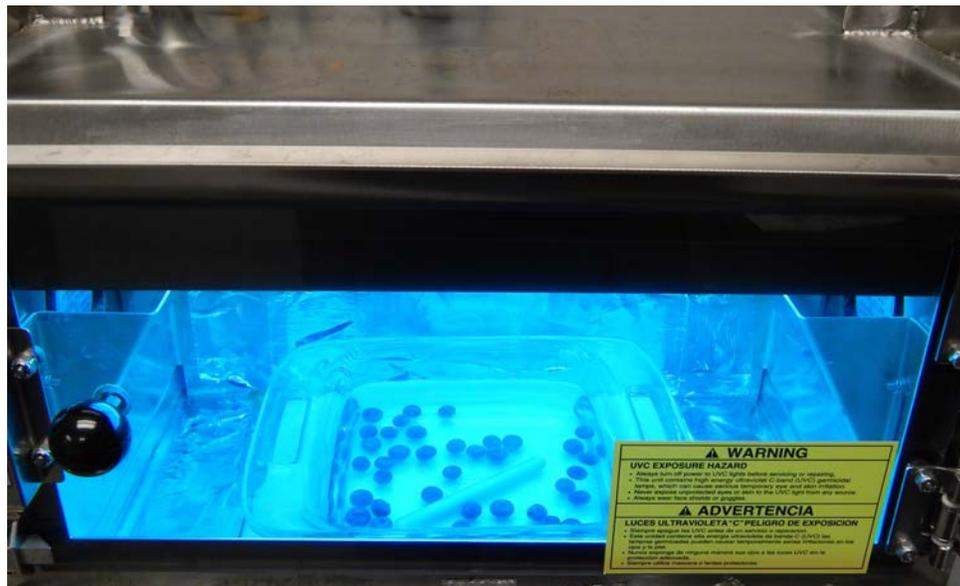
Figure 4.1: Large-scale Water-assisted UV Treatment Setup
