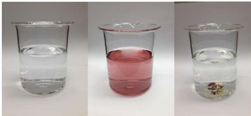
Figure 4.3: Washing Solution in Quartz Beaker. Left to right: DI water, DI water with 2% (v/v) blueberry juice, DI water with 5% [w/w] crush.
