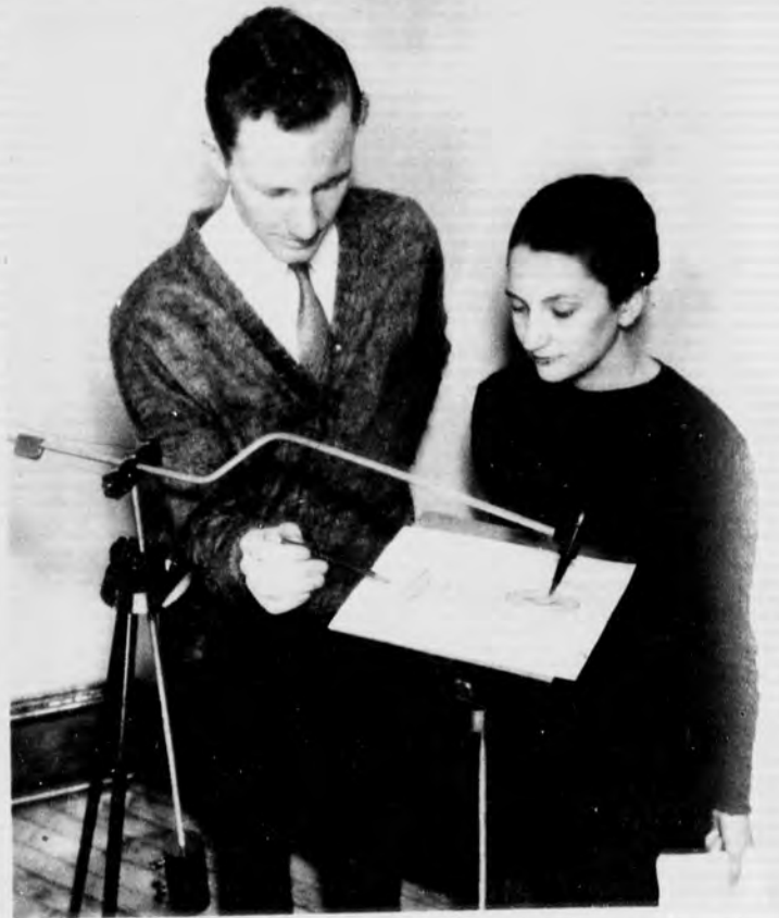
A PRECISION HARMONOGRAPH , believed to be the only one of its kind in the United States, has been designed and built by Milan Fiske, Beloit (Wis.) College junior. The instrument demonstrates compounds of harmonic motions. He has made 10,000,000 different curves with it.
