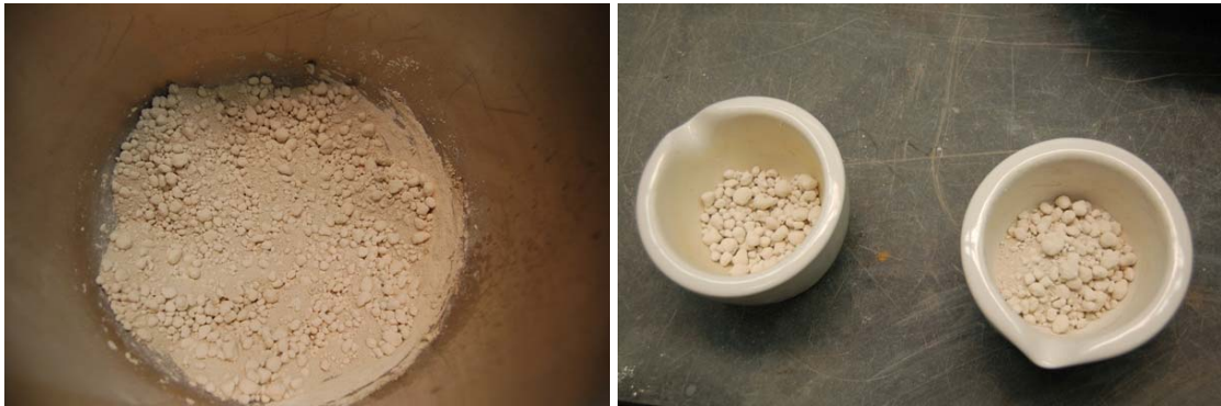
Figure 3.7. Soil Aggregate in Mixture with 50% Kaolinite.
