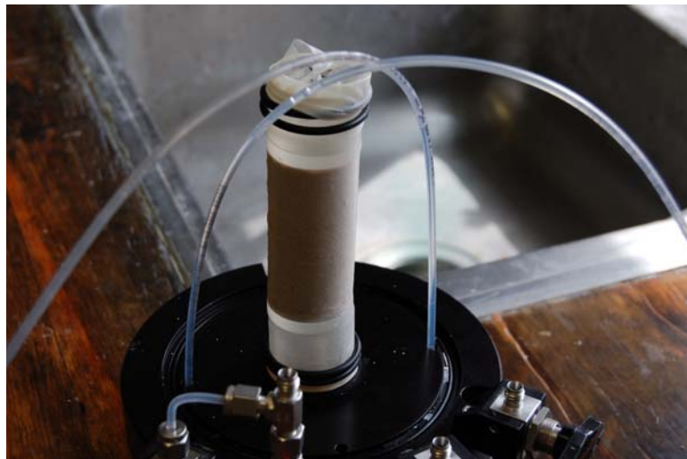
Figure 5.6. Specimen Encased in Membranes and Sealed with “O” Rings
