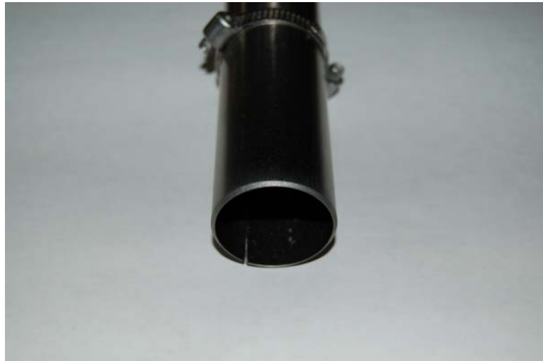
Figure 5.2. Sharpened Edge of Sampling Tube
