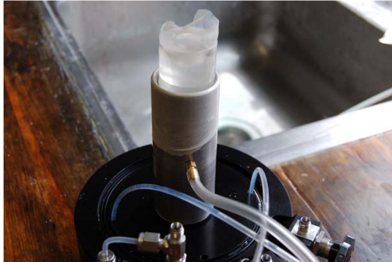
Figure 5.5. Membranes Installed with an Expander
