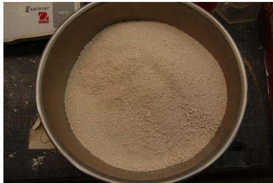
Figure 3.9. Appearance of Sand/Clay Mixture after Grinding.
