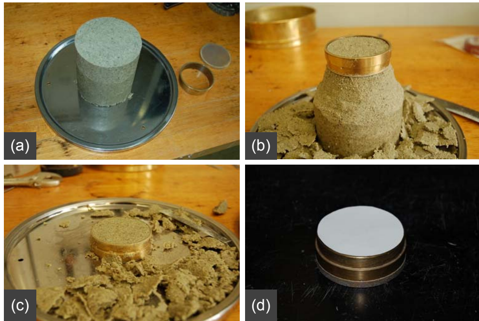
Figure 6.1. Compression specimen preparation procedure; (a) placing the compacted Proctor sample on a turntable, (b) trimming specimen into the consolidation ring, (c) trimming the top and bottom of the specimen flush with the consolidation ring, (d) placing filter papers on the top and bottom of the specimen.
