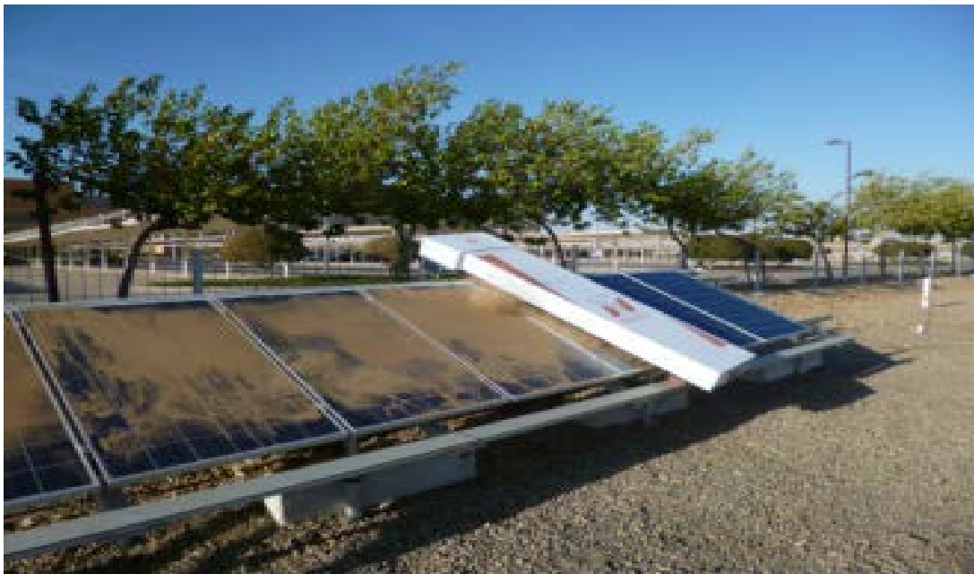
Figure 2.7 Application of the NO Water Mechanical Automated Dusting Device (NOMADD)
