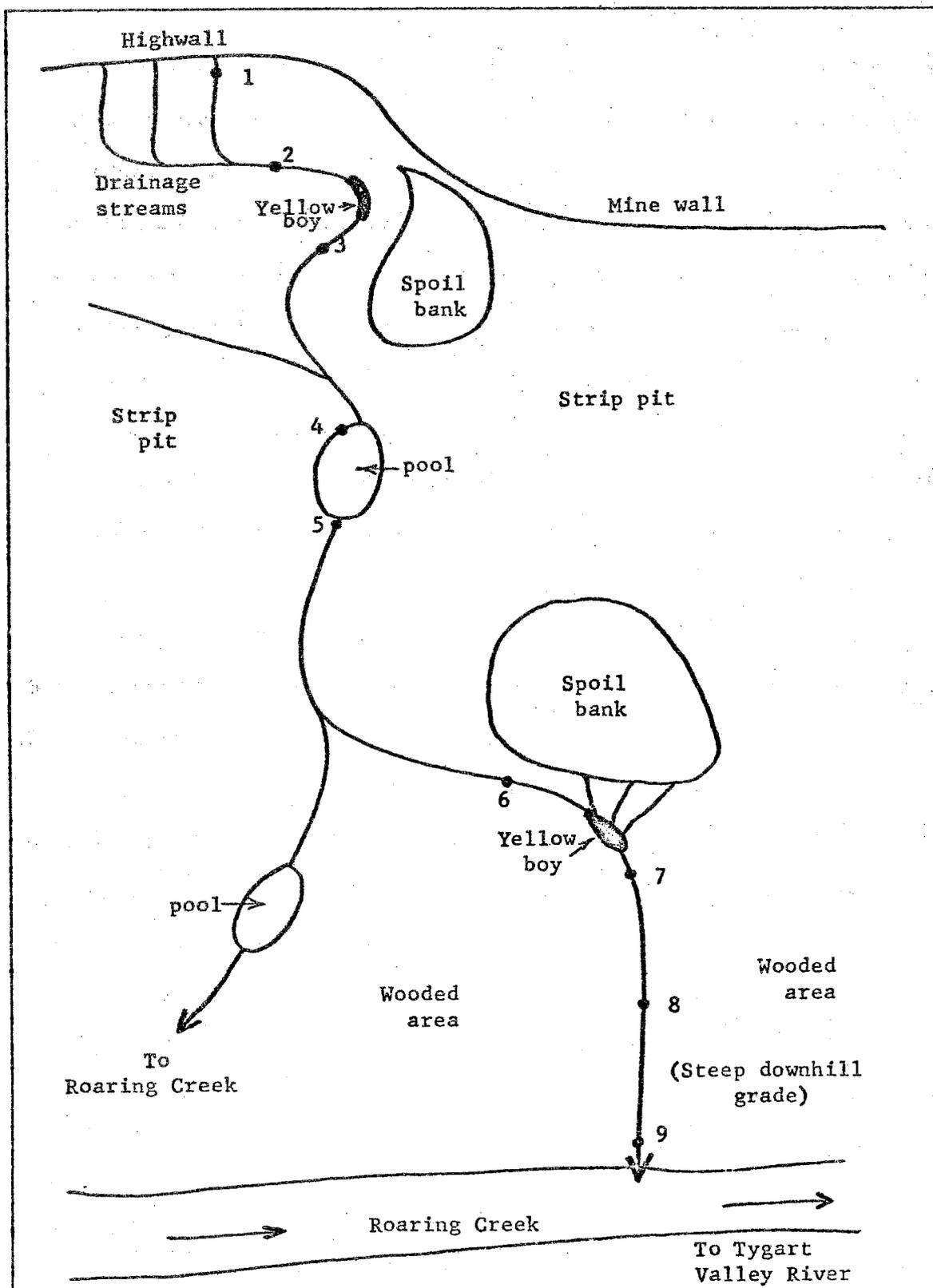
FIGURE 5-10a. Aerial view of drainage through a strip (surface) mine in the Mercer seam near Elkins, West Virginia. The points (•) refer to locations at which samples were collected for laboratory analyses.
