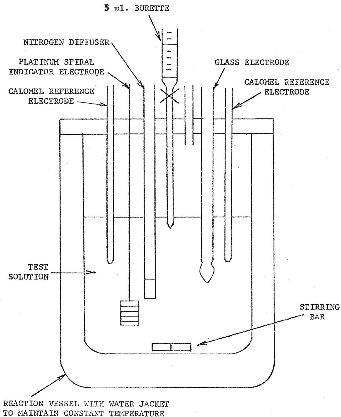
FIGURE 2-15. Experimental apparatus for potentiometric determination of stability constant of sulfato-complex of ferric iron.
