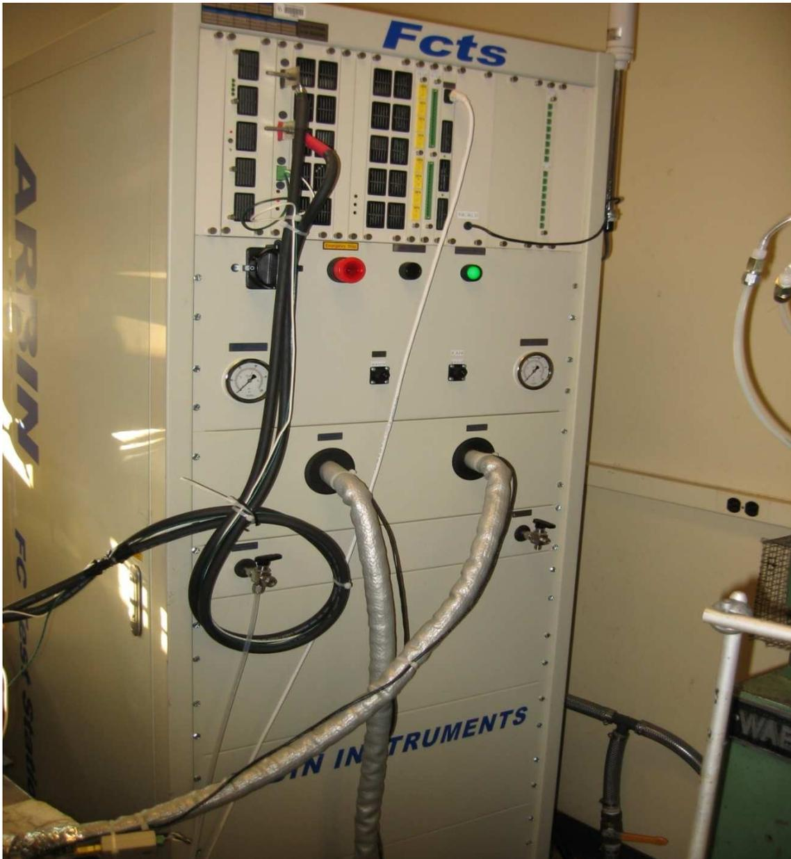
**Figure 7: Arbin Instrument Fuel Cell Test Stand**
