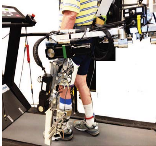
Figure 3.1 The active leg exoskeleton (ALEX) worn by the subjects on their affected extremity during training and treadmill evaluation.
