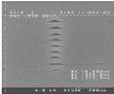
**Figure 2.4:** Cross-sectional SEM of self assembled quantum dots stacked along the growth direction [4].
