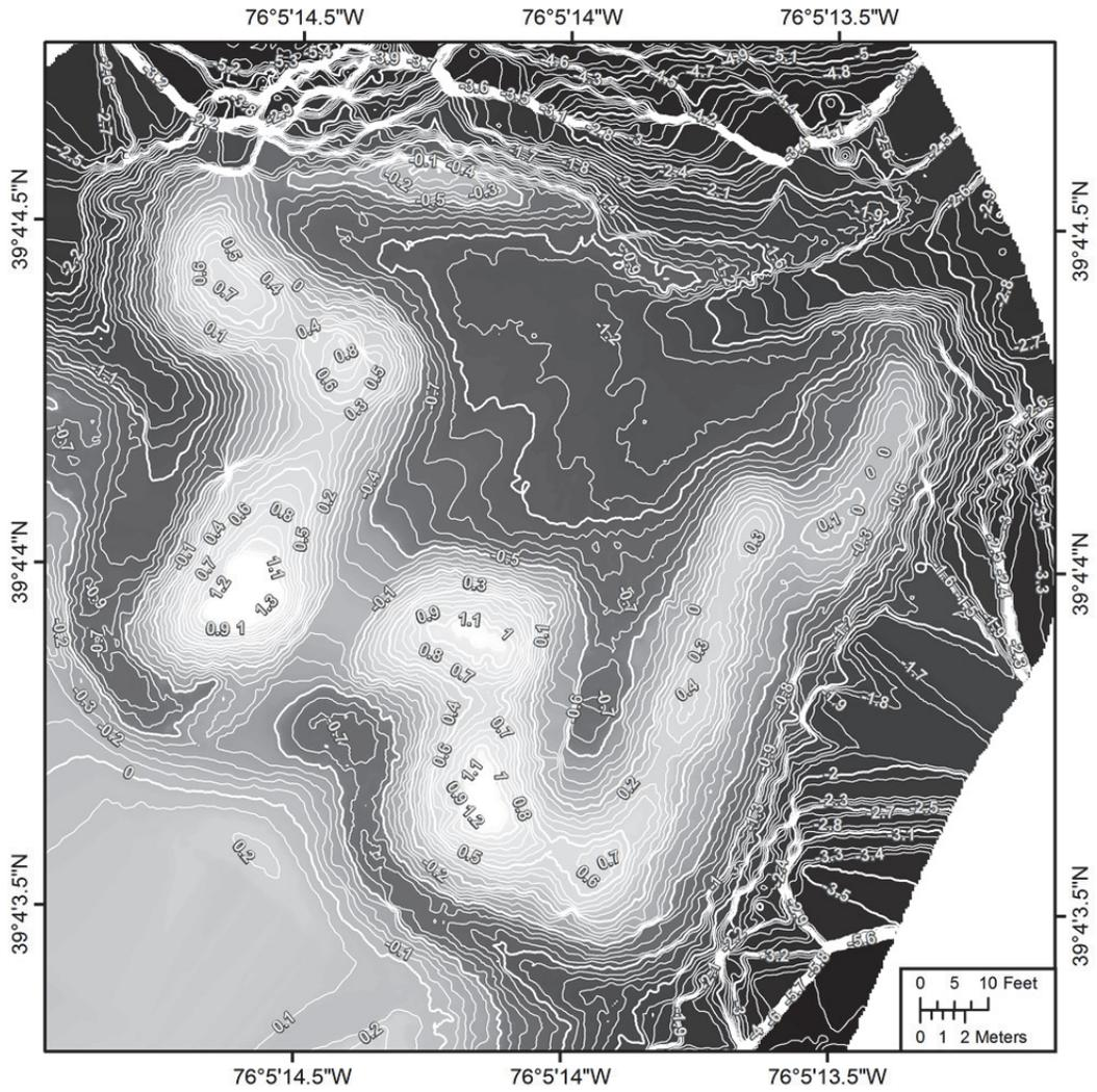
Figure 12: Digital elevation model (DEM) of Fort Point displaying 0.1 m contour lines (white lines) against a shaded background depicting relative elevation.
