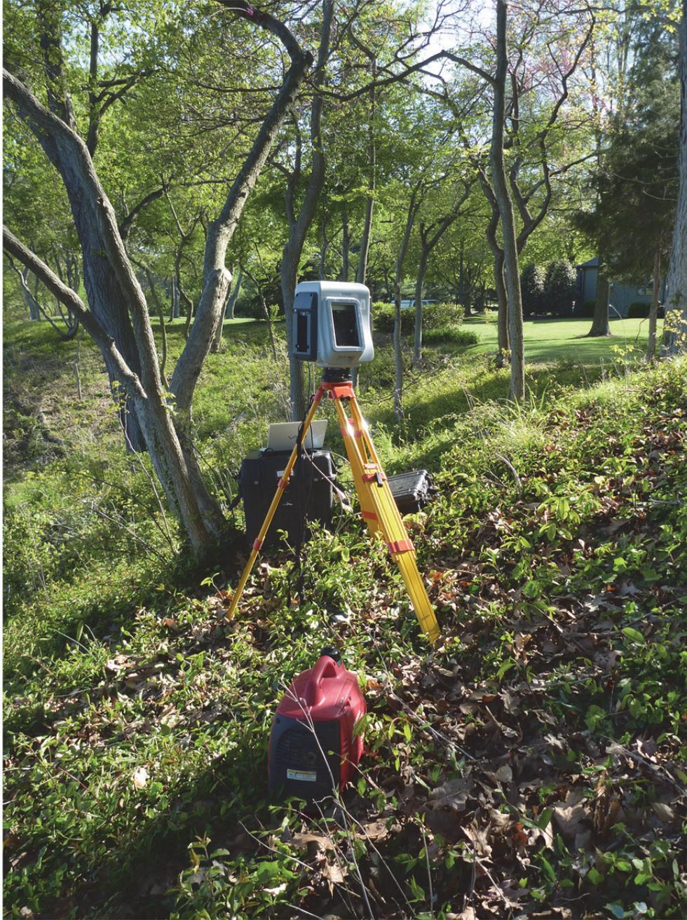
Figure 7: View of TLS in use at Fort Point, showing typical setup. The Trimble GX Advanced Terrestrial Laser Scanner rotates around a fixed axis (tripod), collecting data points which are communicated via a network connection to the laptop and modeled using specialized software.
