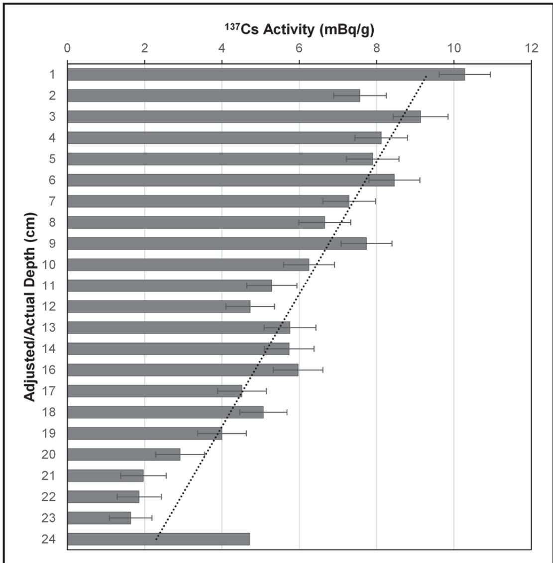
Figure 22: Bar chart displaying  $^{137}\text{Cs}$  activity versus depth below ground surface from Core D at Fort Point. These data suggest post-depositional redistribution of  $^{137}\text{Cs}$ .
