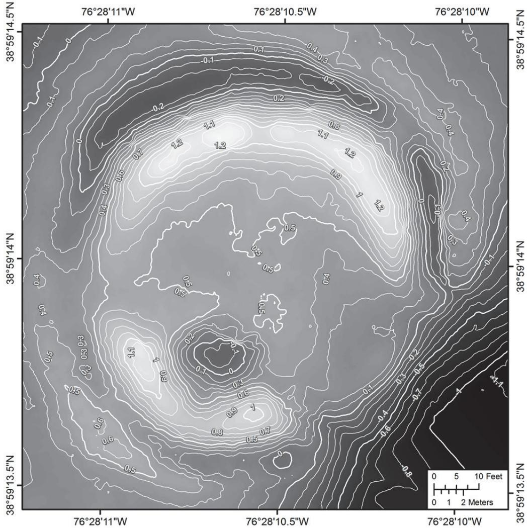
Figure 10: Digital elevation model (DEM) of Fort Nonsense displaying 0.1 m contour lines (white lines) against a shaded background depicting relative elevation.
