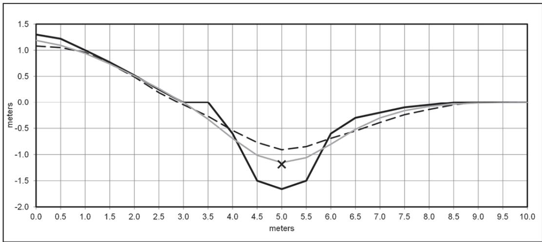
Figure 19: Graph incorporating the 100-yr chronostratigraphic marker determined by  $^{210}\text{Pb}_{\text{ex}}$  dating (black X) into the diffusion model for Profile B at Fort Point, with an estimated initial fort profile (black line), a modeled profile after 100 yrs (gray line), and the actual current topography from TLS data (black dashed line).
