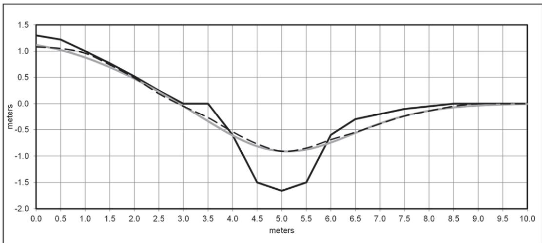
Figure 15: Graph displaying the results of the diffusion model for Profile B at Fort Point with an estimated initial fort profile (black line), a modeled profile after 200 yrs (gray line), and the actual current topography from TLS data (black dashed line). The diffusivity,  $\kappa$ , is  $0.0035 \text{ m}^2 \text{ yr}^{-1}$ .
