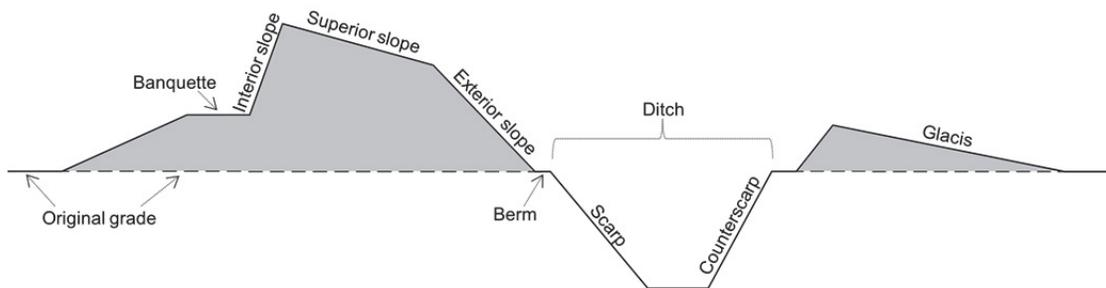
Figure 2: Profile of a typical earthen field fortification, showing the parapet and ditch configuration common to all varieties. Modeled after Mahan, 1862.
