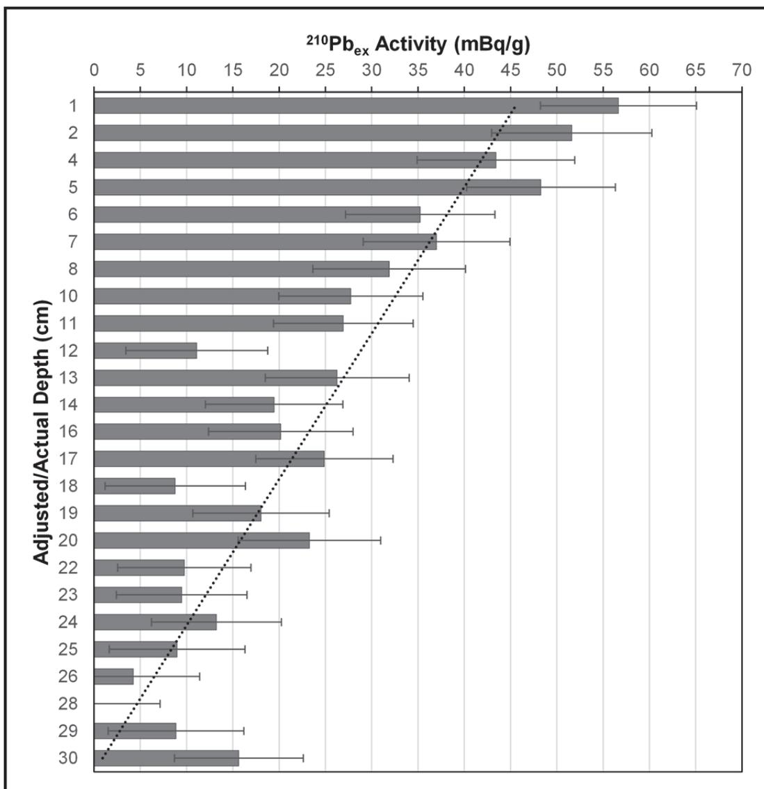
Figure 17: Bar chart displaying  $^{210}\text{Pb}_{\text{ex}}$  activity versus depth below ground surface from Core B at Fort Point. These data suggest the 100-yr chronostratigraphic marker to be located at 27.53 cm.
