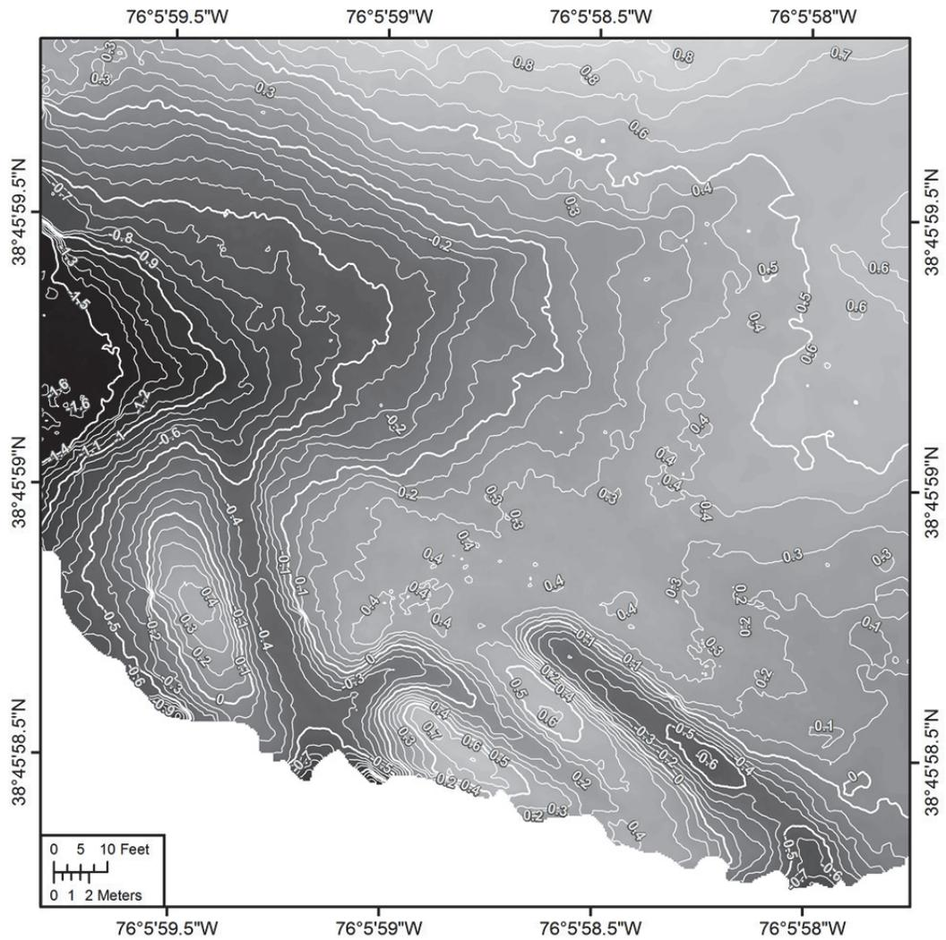
Figure 14: Digital elevation model (DEM) of Fort Stokes displaying 0.1 m contour lines (white lines) against a shaded background depicting relative elevation.
