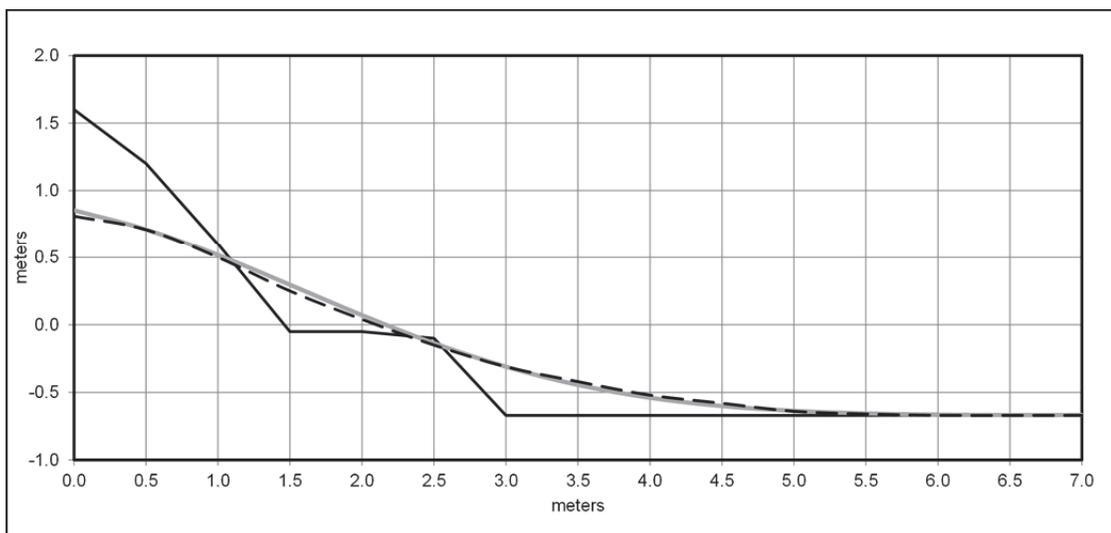
Figure 16: Graph displaying the results of the diffusion model for Profile D at Fort Point with an estimated initial fort profile (black line), a modeled profile after 200 yrs (gray line), and the actual current topography from TLS data (black dashed line). The diffusivity,  $\kappa$ , is  $0.0048 \text{ m}^2 \text{ yr}^{-1}$ .
