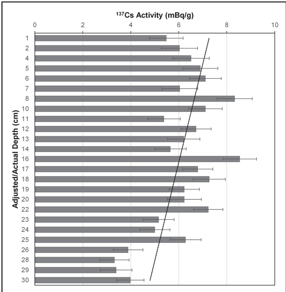
Figure 21: Bar chart displaying  $^{137}\text{Cs}$  activity versus depth below ground surface from Core B at Fort Point. These data suggest post-depositional redistribution of  $^{137}\text{Cs}$ .
