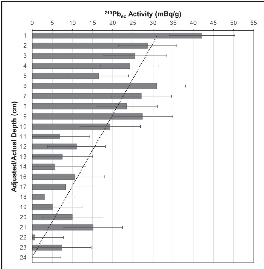
Figure 18: Bar chart displaying  $^{210}\text{Pb}_{\text{ex}}$  activity versus depth below ground surface from Core D at Fort Point. These data suggest the 100-yr chronostratigraphic marker to be located at 23.78 cm.
