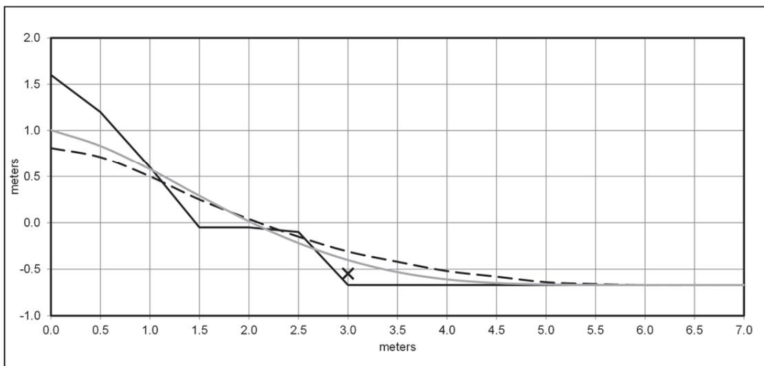
Figure 20: Graph incorporating the 100-yr chronostratigraphic marker determined by  $^{210}\text{Pb}_{\text{ex}}$  dating (black X) into the diffusion model for Profile D at Fort Point, with an estimated initial fort profile (black line), a modeled profile after 100 yrs (gray line), and the actual current topography from TLS data (black dashed line).
