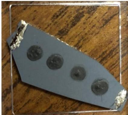
Figure 5-8: Photograph of a coupon (measuring ~1" long) processed with 4 devices of ~8 mm<sup>2</sup> area
